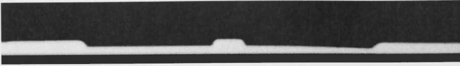
Figure 7.8: Cross sectional optical microscope view of the finished imprinted rib waveguide
