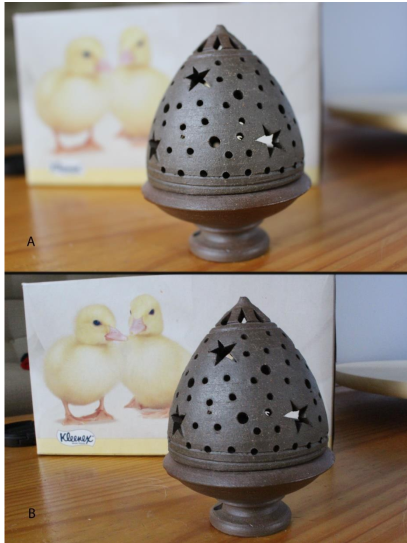
Figure 4 Demonstration of the effect of depth of field. The same scene above is shown when shot using two different camera settings. (A) A relatively high aperture setting creates a shallow depth of field in which only part of the scene is in sharp focus while the rest is blurred. (camera settings: f/4 , shutter speed 1/30 sec). (B) A low aperture setting creates a large depth of field which brings the entire scene in focus (camera settings: f/22 , shutter speed 1/8 sec).
