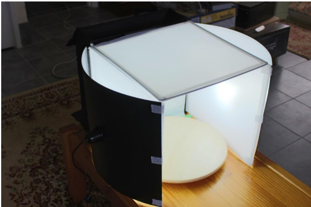
Figure 2 Portable photo studio arranged over a wooden turntable for recording an artefact in 360 degrees under optimal, even lighting.
