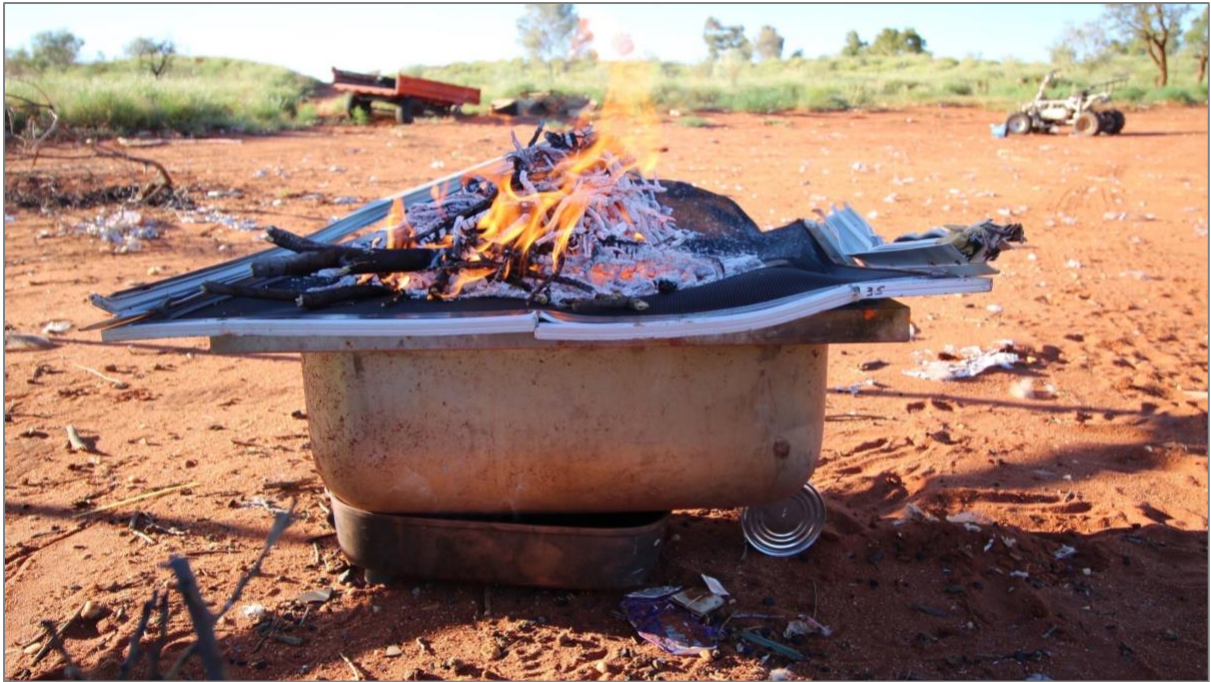
Figure 8.4 Assemblage for burning, filtering and catching ashes
