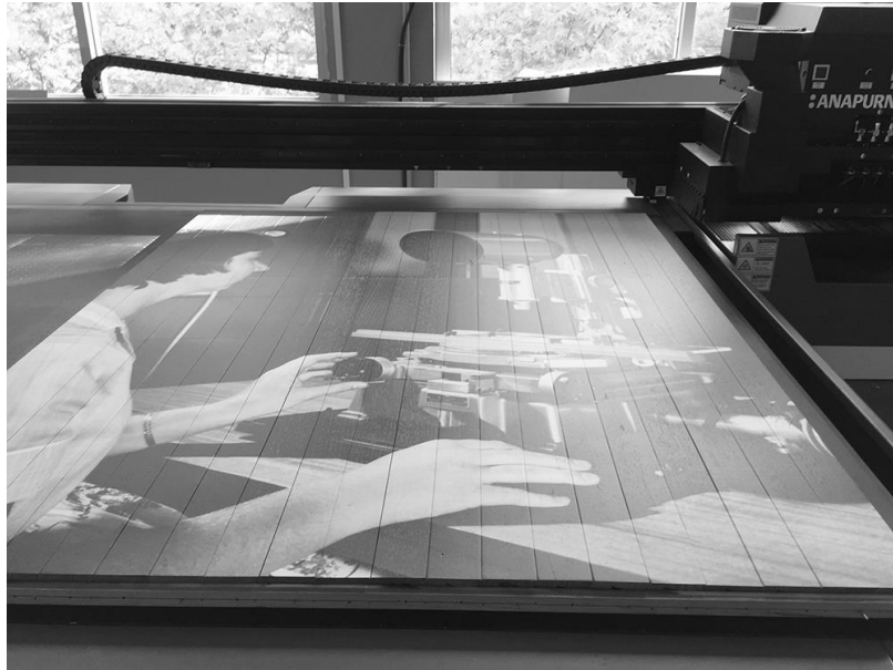
Figure 127: Historical image in the process of being printed on timber slats (image by author)
