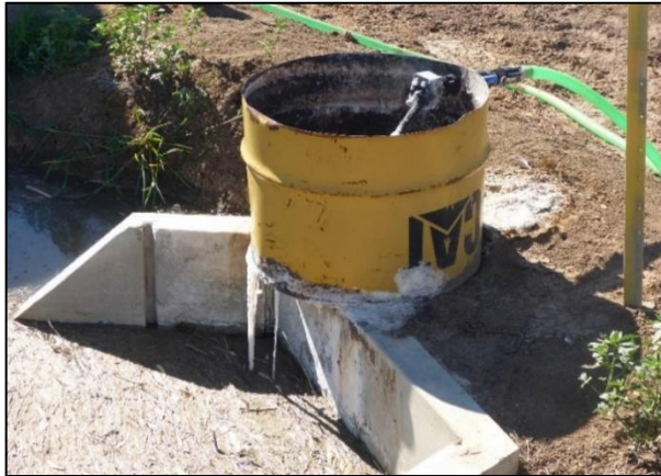
Figure 2.15. Photo of grower-made header tank for regulating the discharge rate from their urea tank. Header tank constructed from half a 44 gallon drum and a valve regulated with an old toilet cistern float switch.
