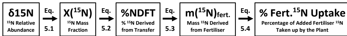
Figure 5.3. Four step calculation of absolute value percentage fertiliser ^{15}\text{N} uptake from IRMS output of relative \delta values.
