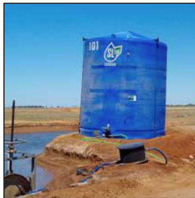
Figure 2.3. Common aqueous urea delivery setup using a large water tank to dispense high concentration urea—N solution into the main irrigation supply channel. Image from SLTEC (2016).
