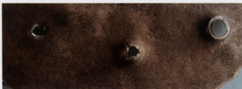
Figure 271. Tested hole-making methods in thin material (back): ( left ) Rostoker's method, ( centre ) punched hole with rupture prongs, ( right ) punched and cut back with abrasive.
