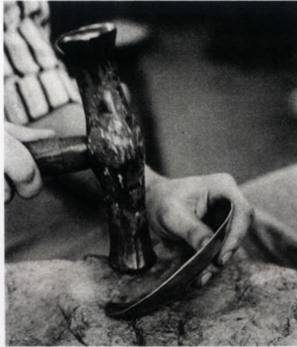
Figure 69. Sinking a disc with a convex hammer-face over a shallow hollow carved into a stump. Source: F. Loyer, The Thames and Hudson Manual of Silversmithing (London: Thames and Hudson, 1980), fig. 40.
