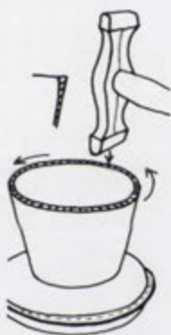
Figure 89. Caulking a vessel's rim by forging it back down into the wall. Adapted from: Smith, Practical Silver-Smithing and Jewelry , fig. 19.
