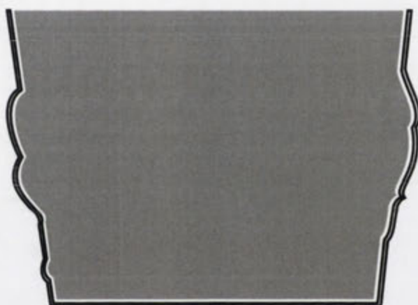
Figure 106. Use of a core to create relief decoration on a ‘Vapheio’ cup. The core, indicated in grey, would be locked into the cup by the relief forms.
