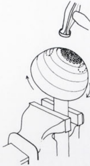
Figure 84. Planishing a hemispherical bowl. The vessel is rotated clockwise (dotted lines show position of finger and thumb, and overlapping hammer blows applied in a spiral or concentric circles. Adapted from: Smith, Practical Silver-Smithing and Jewelry, fig. 69.
