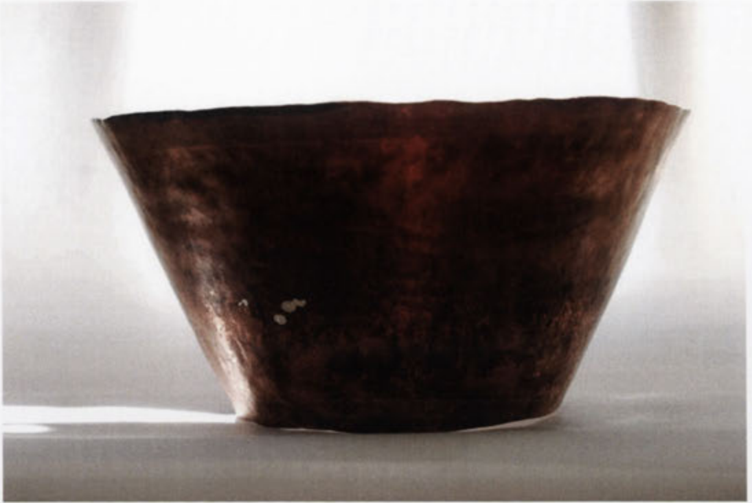
Figure 293. Experiment 3.2: side view. White patches on the lower-left are silver solder which was used to repair tears during the shaping stages.
