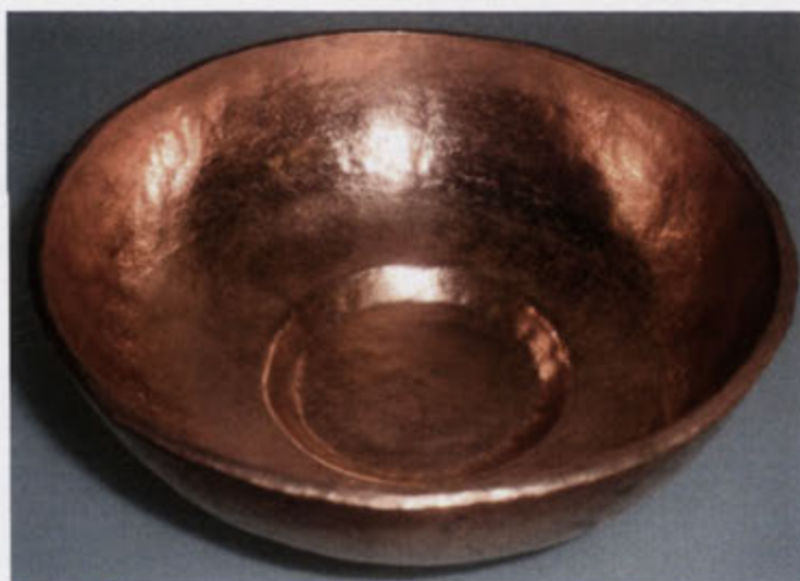
Figure 247. The second bowl made during initial experimentation: the foot is dropped, the rim caulked and the inner surface burnished to a polish.
