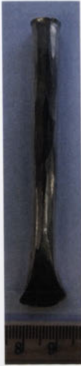
Figure 259. Chisel forged from sterling silver rod. cf. figure 161.
