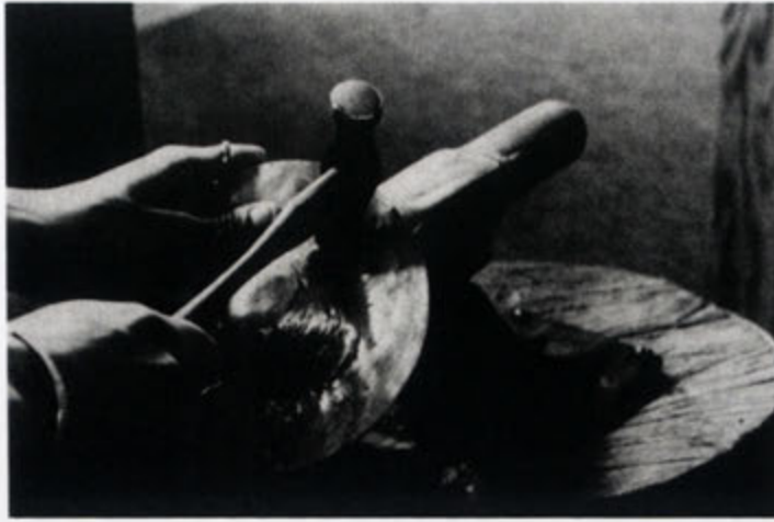
Figure 73. Raising a disc over a steel stake with a steel hammer. In this case the hammer-face is convex. Source: N. C. Humez, Silversmithing: A Basic Manual (Boston: Little, Brown and Company, 1976), 99, bottom.
