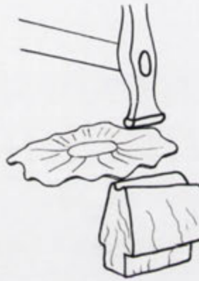
Figure 72. Crimping a disc with a cross-peen hammer into a wooden crimping stake. Source: E. Brepohl, The Theory and Practice of Goldsmithing , trans. Charles Lewton-Brain (Portland: Brynmorgen Press, 2001), fig. 6.12.
