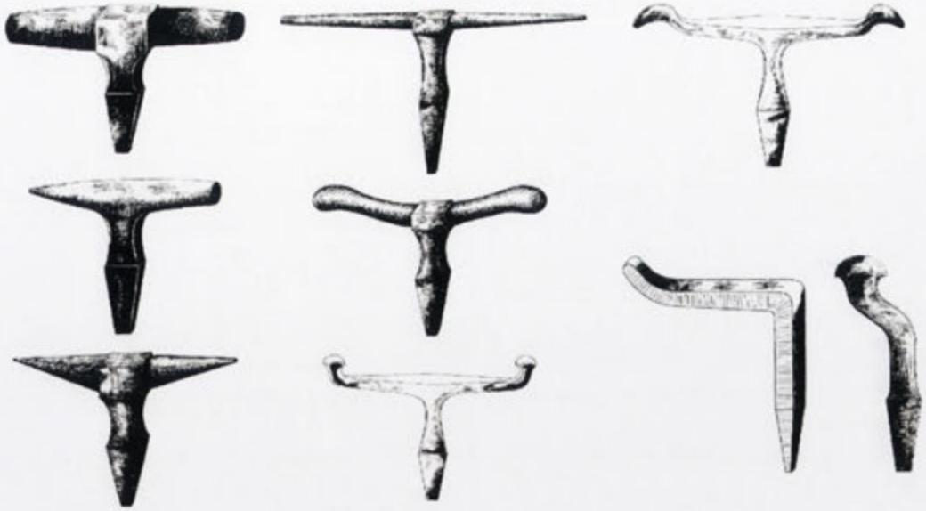
Figure 82. A selection of steel raising stakes. Shapes range from simple, straight forms (left) to increasingly complex forms (right). Adapted from: Der Silberschmied: Lehr- und Handbuch , (Stuttgart: Ruhle-Diebener-Verlag, 1982), figs 24-31.
