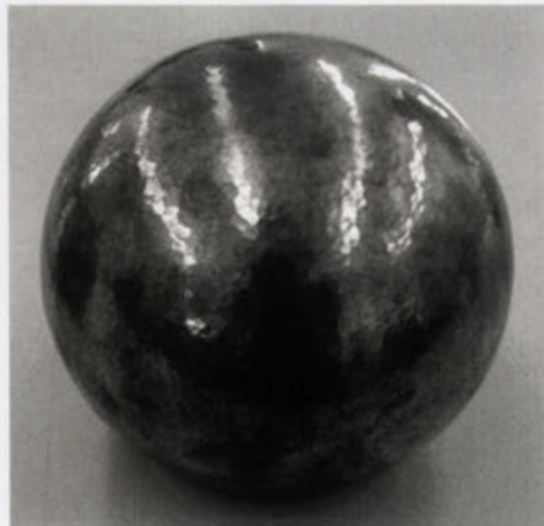
Figure 87. A hammered copper sphere with the faceted surface characteristic of planishing.
