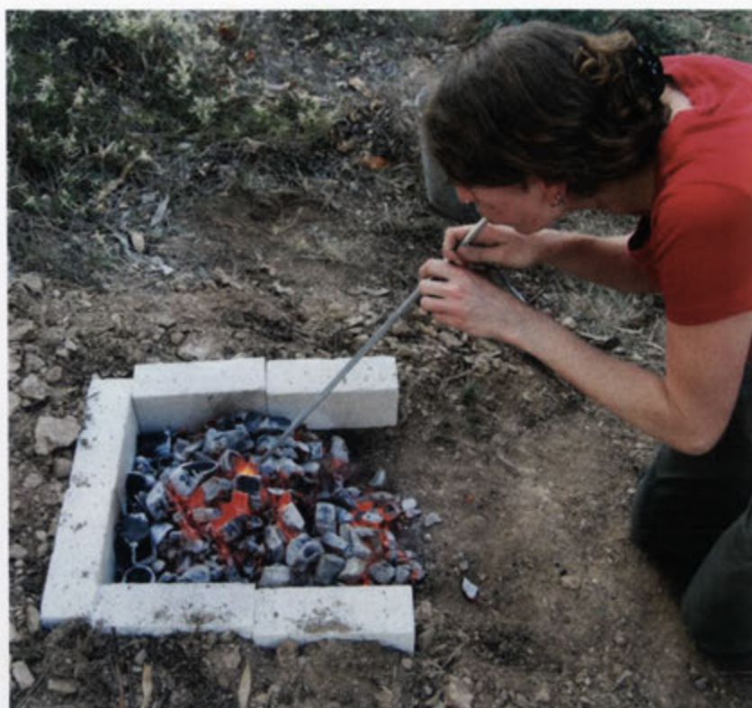
Figure 262. Annealing a billet buried in the hearth using an aluminium blow-pipe.
