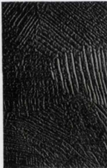
Figure 96. Metallographic image of the Egyptian bowl shown in Figure 95 at 4x magnification. The fact that the dendrite and grain structures are intact shows that the vessel was made by casting with no subsequent hammering. Source: H. E. Winlock, “An Egyptian Flower Bowl,” MMS 5, no. 2 (1936): fig. 3.
