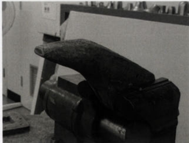
Figure 81. A wooden raising stake held in a vice bolted to a wooden stump.
