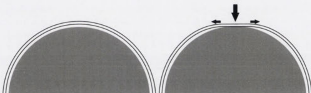
Figure 101. Hammering a vessel over a core. The material on either side of the hammer blow ( large arrow ) would be forced to bow outwards ( small arrows ) and the material under the hammer would be planished thinner, thus stretching it.
