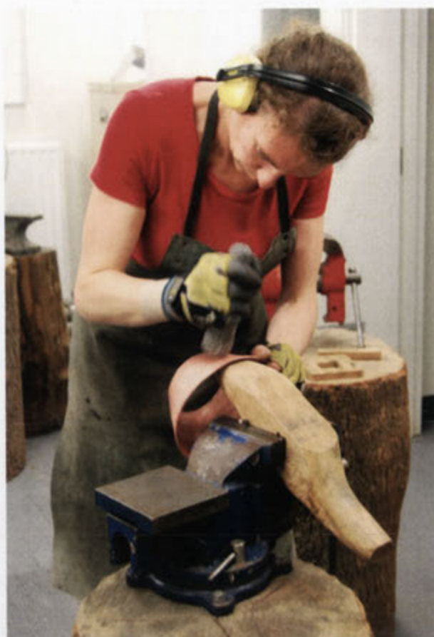
Figure 266. Raising a hydria-section with a granite pestle over a wooden stake.
