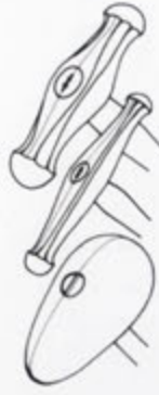
Figure 71. Modern hammers suitable for sinking: (top to bottom) heavy and light steel hammers, wooden pear-mallet. Adapted from: K. Smith, Practical Silver-Smithing and Jewelry (London: Studio Vista, 1975), fig. 8.
