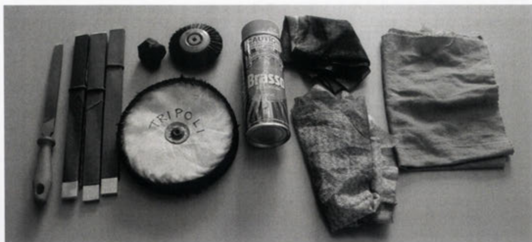
Figure 88. A typical set of equipment for polishing a hammered vessel: (left to right) medium-grade steel file; 400, 600 and 1200 grade emery paper wrapped around aluminium flat-bar; tripoli polish with a nylon-bristle wheel and calico buff; metal polish; rags for cleaning; polish-impregnated felt cloth.
