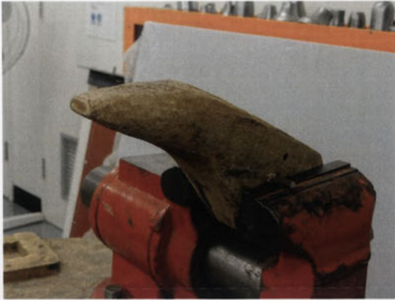
Figure 257. Hardwood stake held in a vice used for raising.
