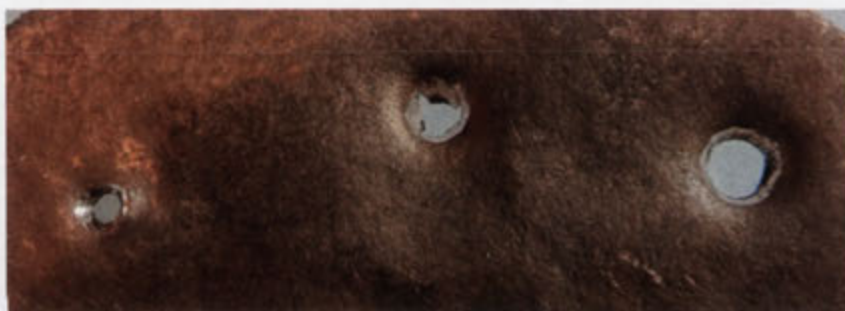
Figure 270. Tested hole-making methods in thin material (front): ( left ) Rostoker's method, ( centre ) punched hole with rupture prongs, ( right ) punched and cut back with abrasive.
