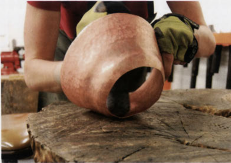
Figure 265. Shaping the bottom-end of a hydria-section after a hole was cut in the base of the concave form.
