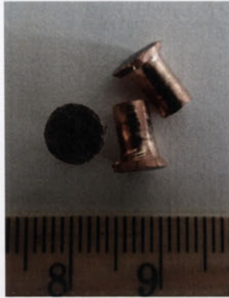
Figure 275. Copper rivets with the first head formed.
