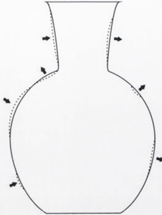
Figure 86. Adjusting the profile of a vessel: high and low spots in the vessel's profile (indicated by broken lines) are brought down by tapping the surface and brought out with localised planishing.
