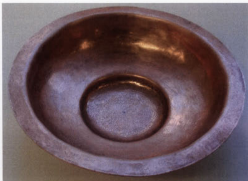
Figure 246. The first copper bowl made during initial experimentation: the foot is dropped, the rim folded out and the inner surface burnished to a polish.
