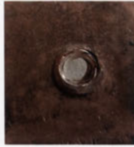
Figure 272. Rostoker's method for hole-making tested on 2 mm copper sheet.
