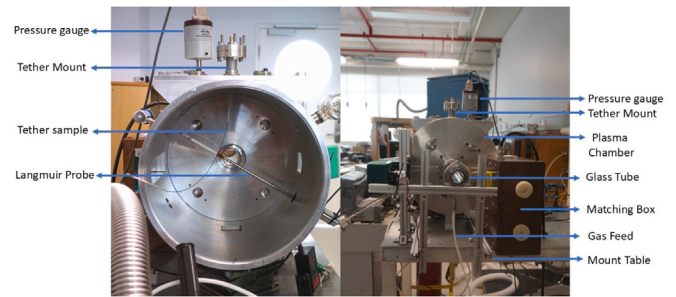
Fig. 1. The plasma chamber setup at the ANU SP3 Laboratory. Left: Internal view of the plasma chamber setup with a tether sample mounted on the chamber ceiling and a Langmuir probe placed perpendicular to incoming plasma, Right: External view of the plasma chamber with connected glass tube and matchbox capacitor.
