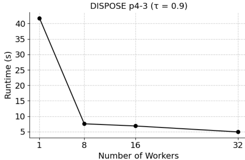
Figure 5.10: Relationship between the number of workers and runtime (seconds) for DISPOSE p4-3 with a probability threshold of \tau = 0.9 . The depths at which valid plans were found are: 28 (1 worker), 9 (8 workers), 8 (16 workers), and 9 (32 workers).
