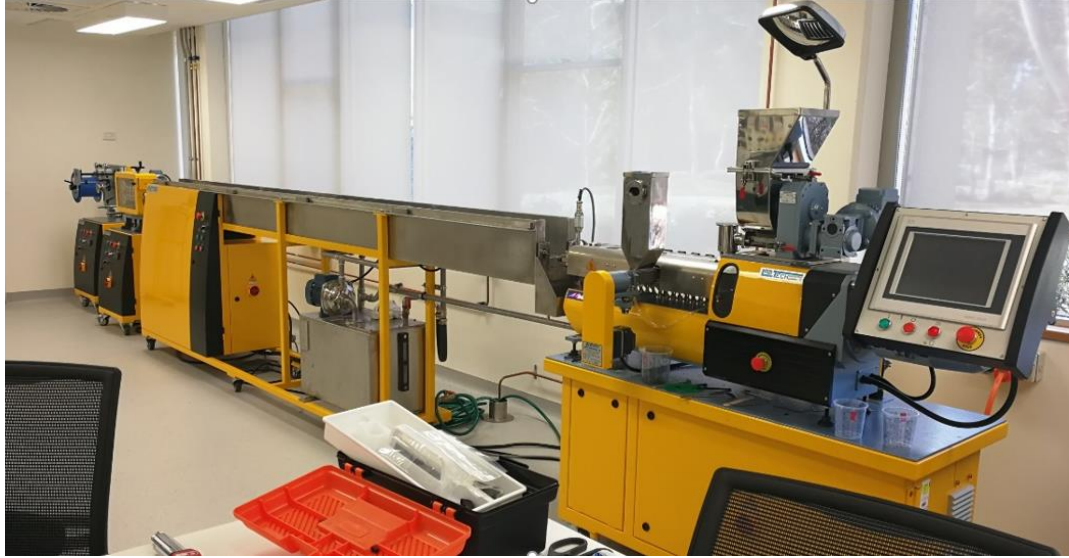
Figure 3.11 The industrial co-rotating twin-screw extrusion line LTE16-44.
