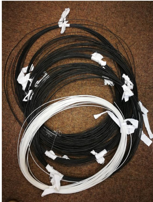
Figure 3.12 The neat PLA and PLA composite filaments with varying CF contents.
