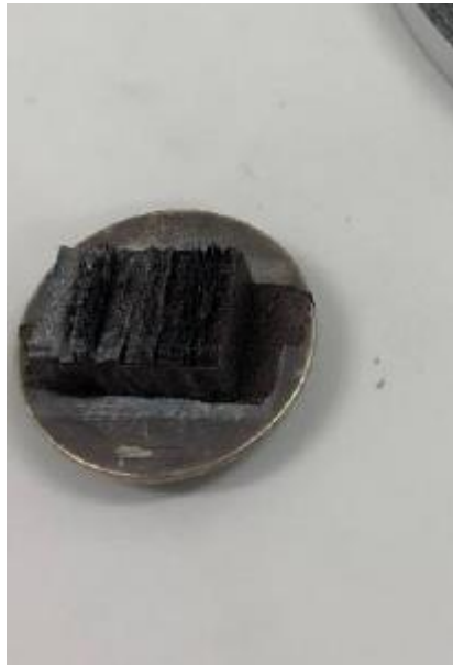
Figure 3.22 The stub fixed samples with gold coating for the fractural observation.
