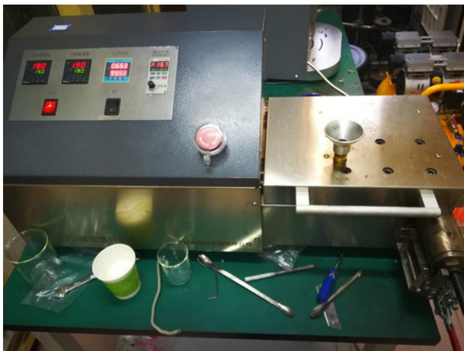
Figure 3.8 The lab-scale miniature twin screw extruder WLG10.
