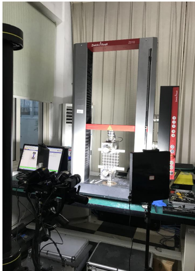
Figure 3.18 The full-field deformation test via a 2D DIC system during the tensile test.
