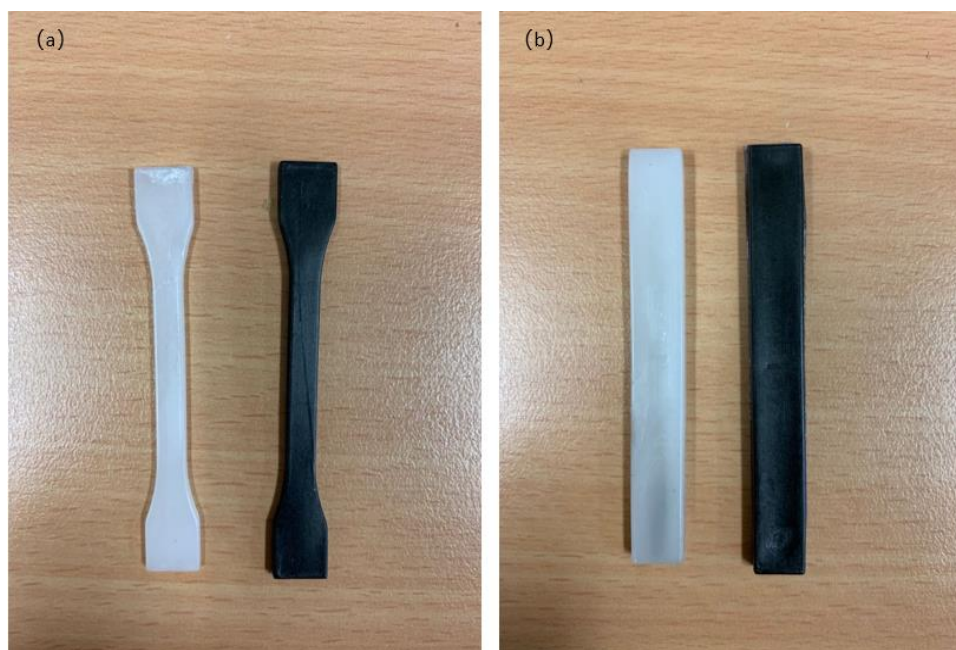
Figure 3.10 Injection molded samples for (a) tensile test and (b) flexural test.
