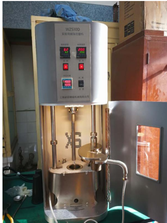
Figure 3.9 The lab-scale miniature injection molding machine WZS10D.
