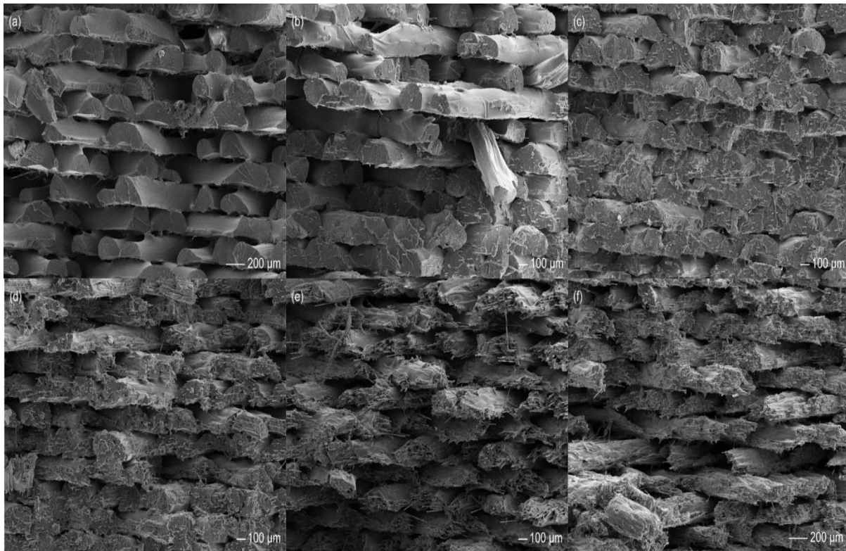
Figure 5.10 The SEM fractural interfaces of CF/PLA composites with (a) 0 wt% CF, (b) 2.5 wt% CF, (c) 5 wt% CF, (d) 7.5 wt% CF, (e) 10 wt% CF and (f) 15 wt% CF at \times 100 magnification.
