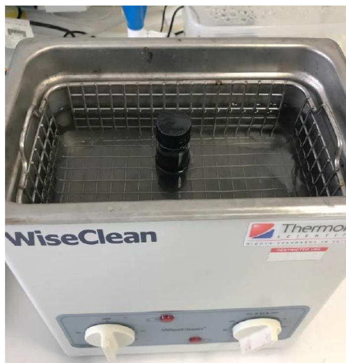
Figure 3.6 The homogeneous dispersion of CNTs in the ethanol solution via ultrasonication.
