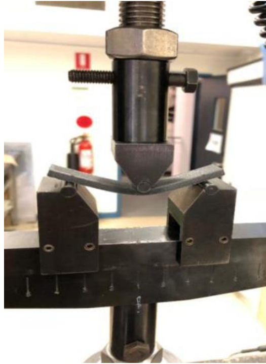
Figure 3.16 The setup of three-point bending for the flexural test.
