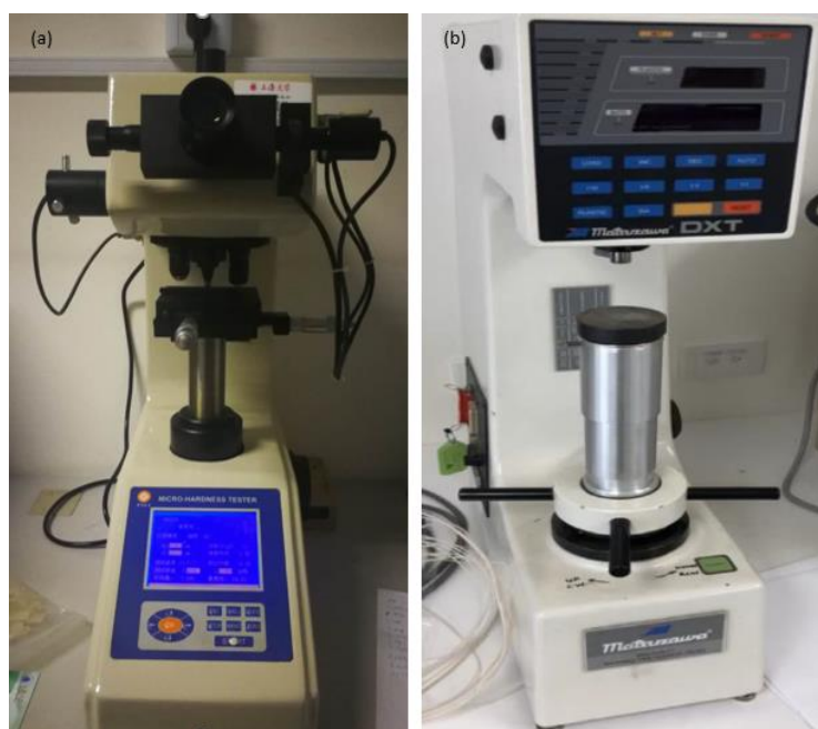
Figure 3.17 Two types of hardness testers: (a) Vickers tester for chapter 4 and (b) Rockwell tester for chapter 5.
