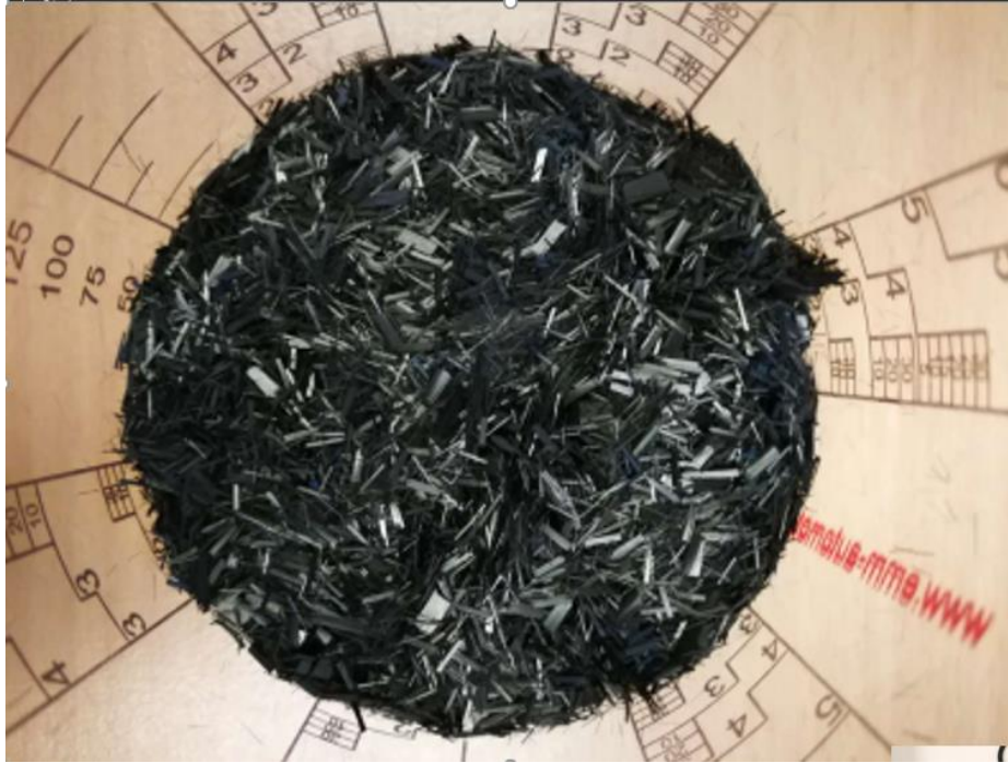
Figure 3.1 The chopped CF with the average length of 4.6mm.
