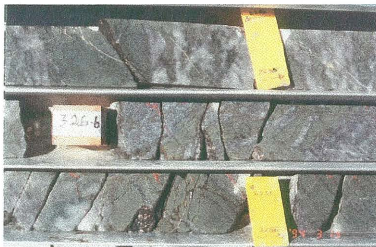
Figure 5.5 – Sheeted quartz veins in drillcore (hole #HD7B, 326.6m). Au values are 37 – 41ppm (Rangott & Bird, 1994).
