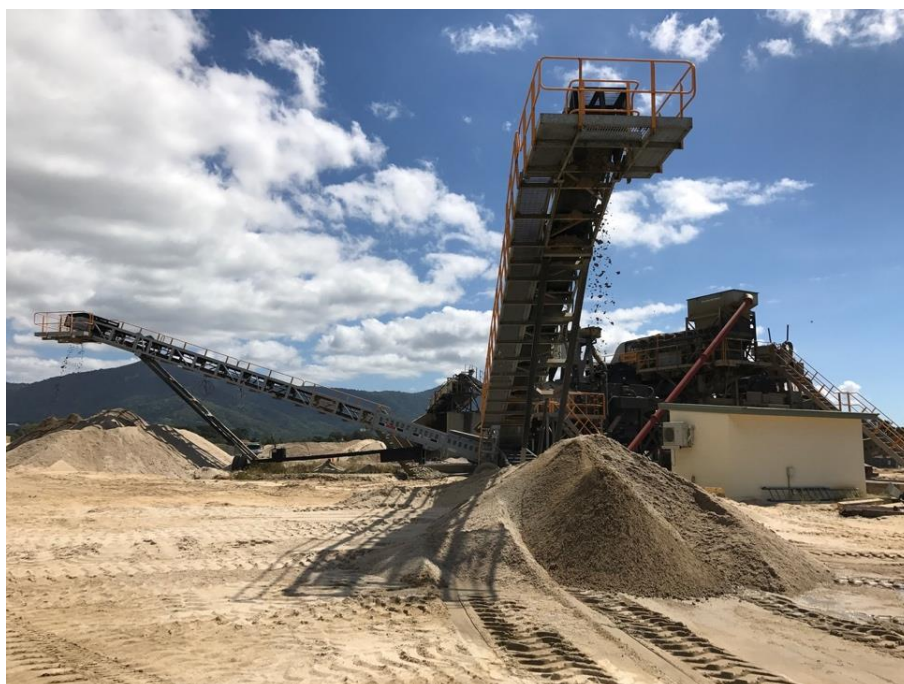
Plate 4. Resource recovery plant at a landfill 110 in the Barron River floodplain, north of Cairns in Queensland. The offshore fines were to come onshore from a shipping channel expansion in the Great Barrier Reef Marine Park. As they contained pyrite, it was necessary for them to be either alkali-treated or interred below the lowest seasonal groundwater level where they would remain anoxic. (Photograph by author, 2019).
