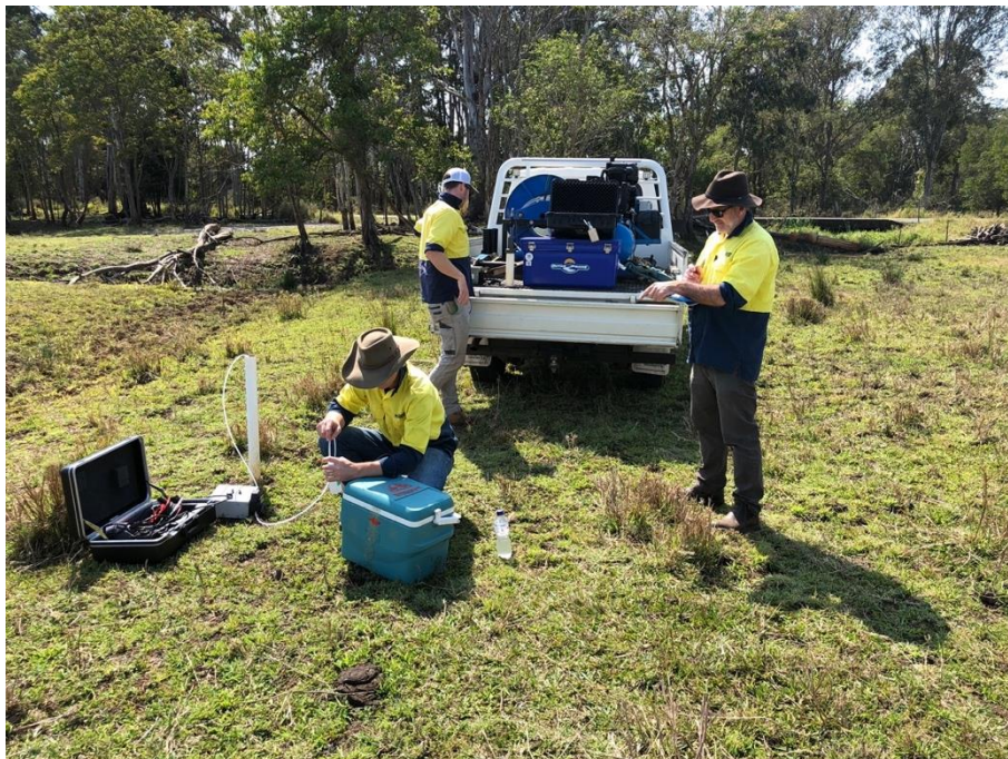
Plate 14. Low flow groundwater testing in the matter of Maroochy Sands v Sunshine Coast Regional Council (2017). This dispute involved a proposed sand mine in a floodplain where the substrate exhibited a high fines concentration. The presence of these fines was to effectively curtail the production rate as settlement times increased. The application was withdrawn. (Photograph by author, 2017).
