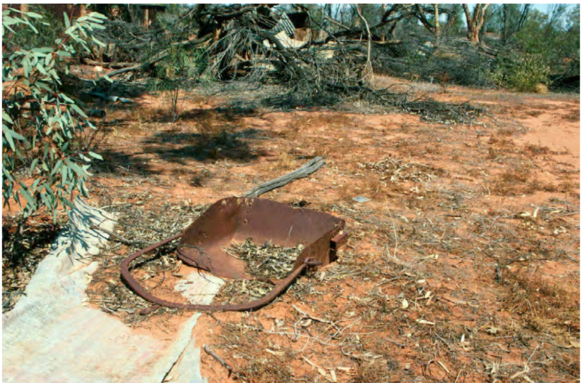
Fig 4.11: Scoop dragged by horse or camel in digging the Paradise well. 1997
