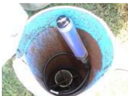
Figure 7.2 shows the pressure transducer groundwater level gauge in a bore. Source: Department of Infrastructure, Planning and Natural Resources
