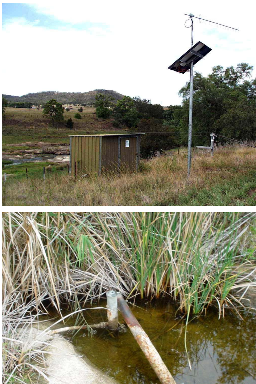
Figure 7.5 Location of the Wybong stream gauge (station #210040) and Pressure sensors that measure stream height
