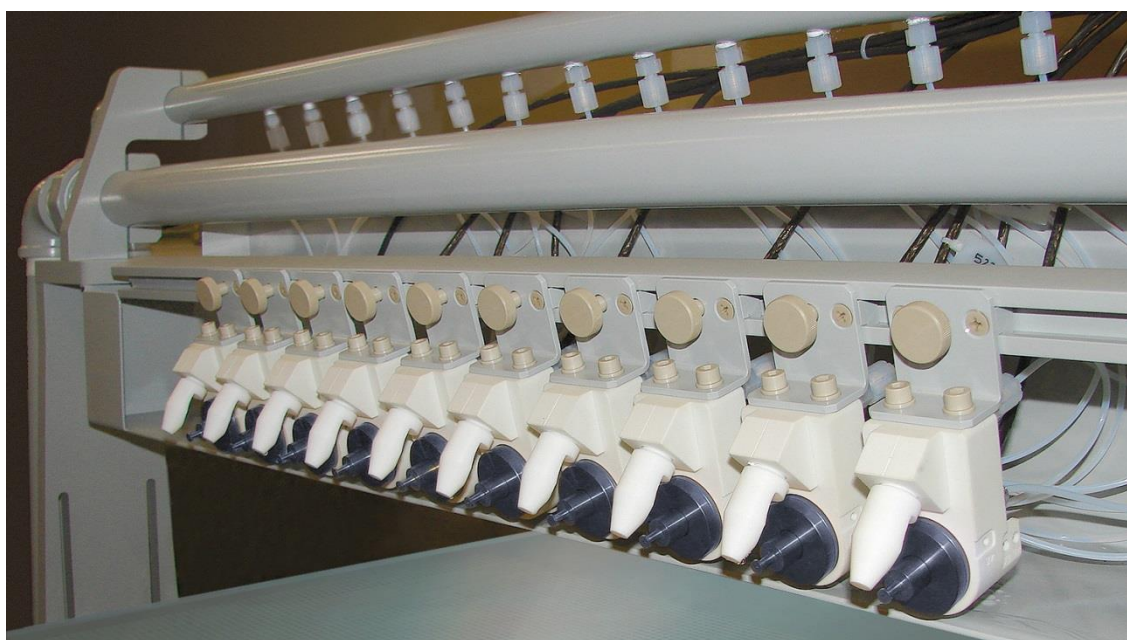
Figure 6.1 Sono-teck's array system of spray pyrolysis nozzles designed to deposit uniform transparent conductive oxide (TCO) layers for mass production of TCO coated glass substrates for thin film solar cell manufacturing (photograph from Sono-Teck Corporation).
