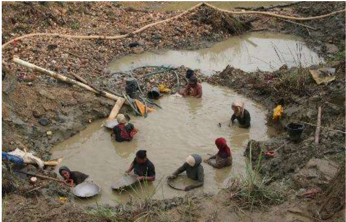
Figure 3.14 Panning activities in a dompeng hole after the washing carpet process
