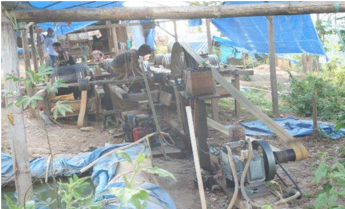
Figure 4.1 A set of tromol machine with ground tailings. Miners use tarpaulins to collect and recycle water from the machine. They can also carry out further panning on the tailings
