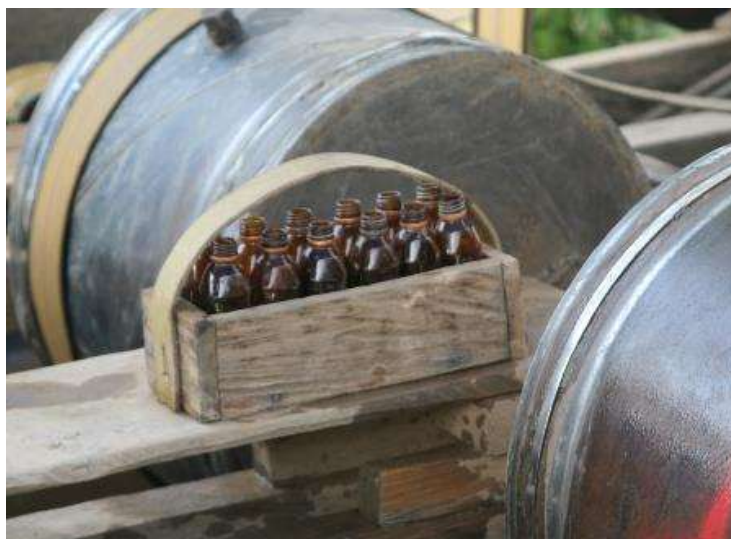
Figure 4.2 The small drink glass bottle for storing mercury tromol machine (top). A wooden carrier for transporting bottles of mercury (bottom)
