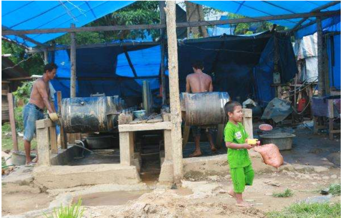
Figure 3.8 This tromol machine belongs to William in Padambila mining site, used for grinding tailings Tromol Machine ( Mesin Tromol ): Mill, Centrifuge and Mercury
