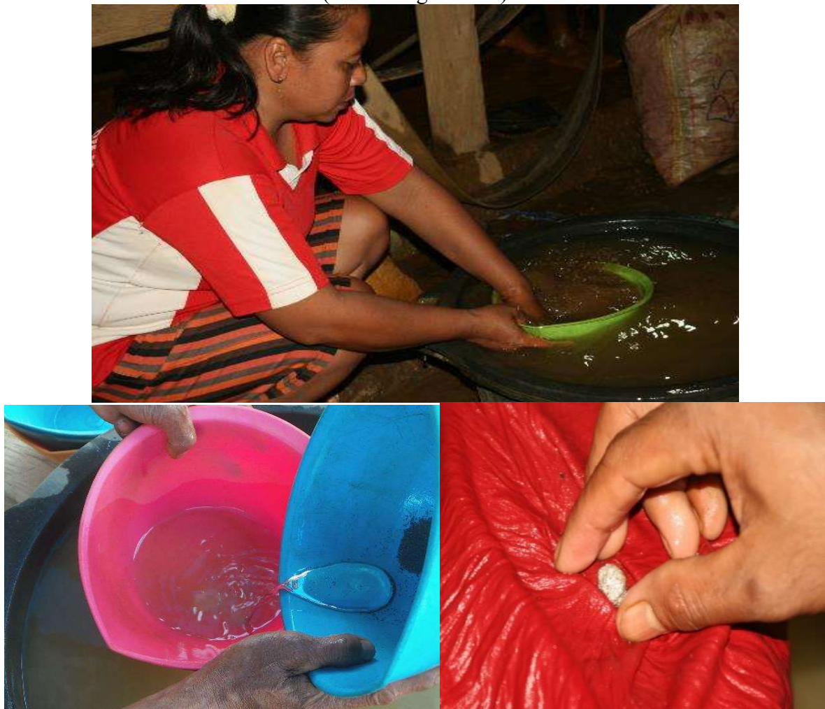
Figure 4.3 Matoyong process: to whisk materials together (central upper). To sift liquid amalgam and to squeeze amalgamated materials forming a gold amalgam (left and right down)
