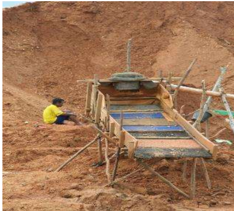
Figure 3.7 Asbuk/kato /sluice box with carpet attached to catch gold flux
