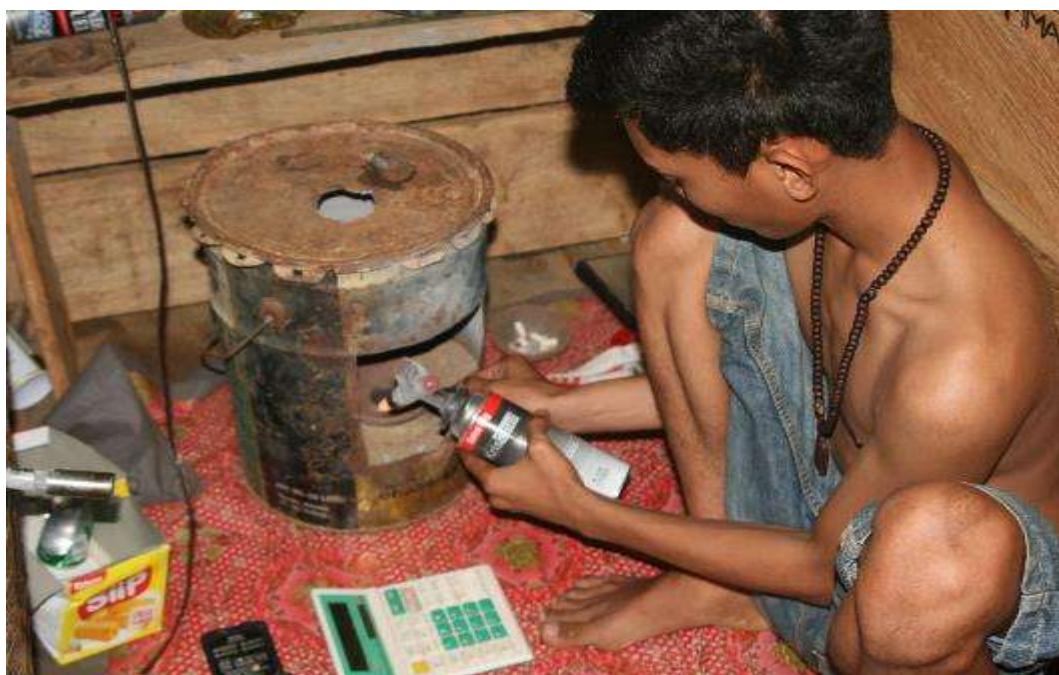
Figure 4.4 The boy burning the amalgam using a hand-held gas burner
