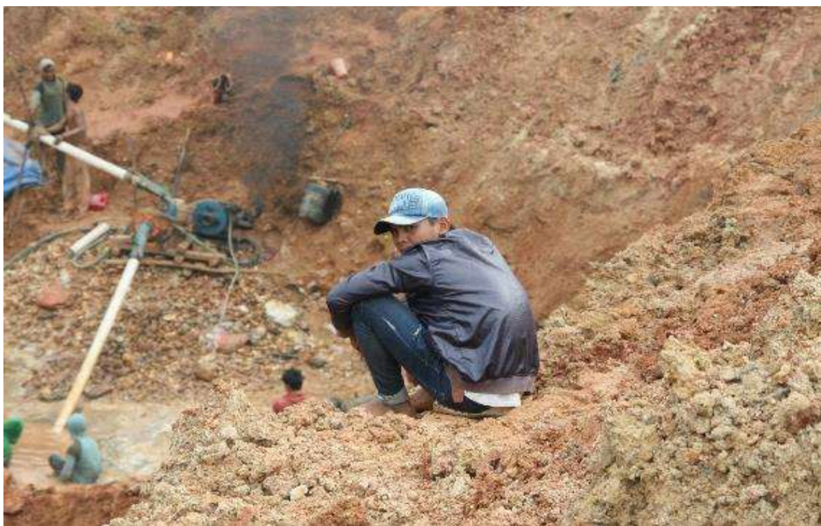
Figure 3.6 Dompeng sluicing activities. The dompeng machines suck the water and distribute it through the pipes and hoses
