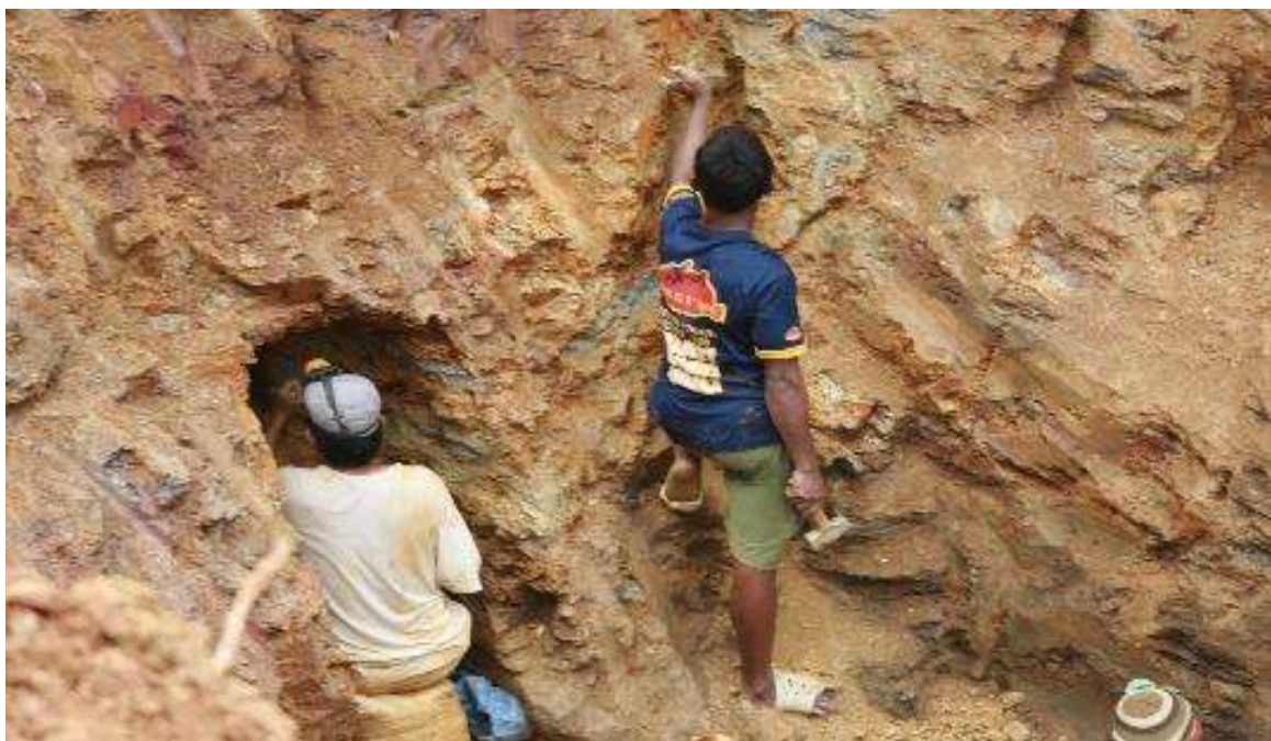
Figure 3.10 A horizontal rat hole where individual miners can dig materials
