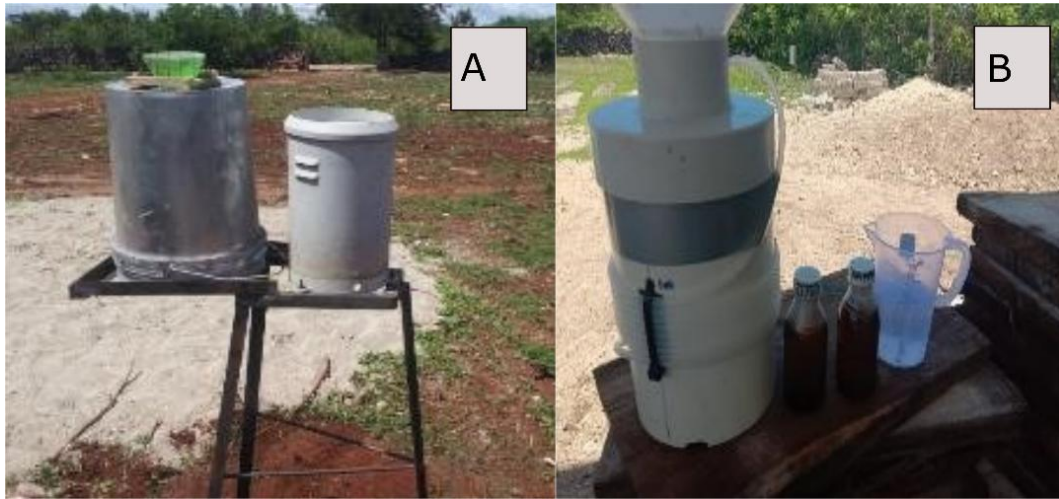
Figure 5.2. A) Rain accumulation sampler used in 2016 and 2017; B) Rain accumulation sampler used to collect weekly composite samples in 2019–2020
