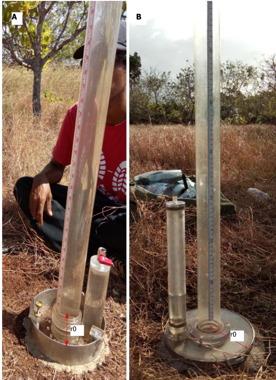
Figure 4.5. A) Ponded disc permeameter setup; B) Unsaturated disc permeameter setup (infiltration with -40 mm negative supply potential). r_0 (the disc radius) is delineated on each permeameter.
