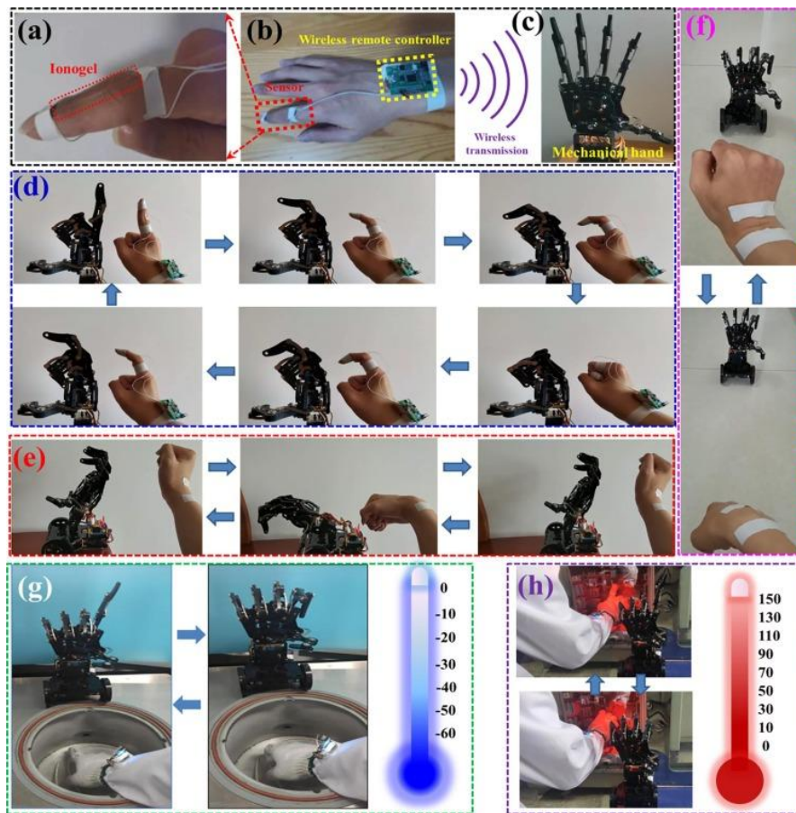
Figure 1. 4. The real-time wireless human–machine interface control system. a-c) Schematic of the system. The response of ionogel based sensor from hand motion is first real-time captured and converted to the digital signal, and then the data is real-time wireless transferred to a mechanical hand. d-f) Human hand gesture recognition and mechanical hand real-time response and reconstruction. g) and h) Human-machine Interface under -60\text{ }^{\circ}\text{C} and 150\text{ }^{\circ}\text{C} . 152 Copyright 2022. Reproduced with permission from Elsevier.
