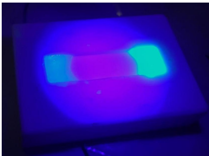
Figure 3. 8. Photocured DVE-3/tetrathiol samples (1:1 ene: thiol in functionality) in the presence of CsPbBr 3 QDs/Iod (left) and CsPbBr 3 QDs/EDB (right) (CsPbBr 3 : 0.5 wt%; Iod: 0.5 wt%; EDB: 0.5 wt%) upon exposure to LED@410 nm (110 mW cm -2 ).
