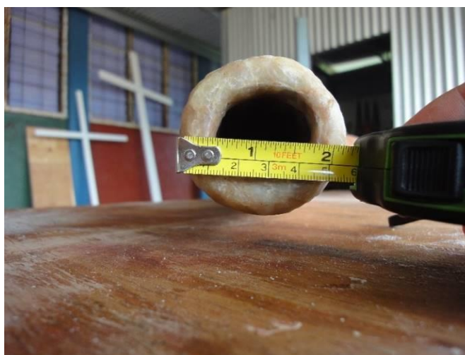
Figure 3.57: Beeswax was added to the mouthpiece to make it soft to the mouth and to adjust the size of the internal diameter
