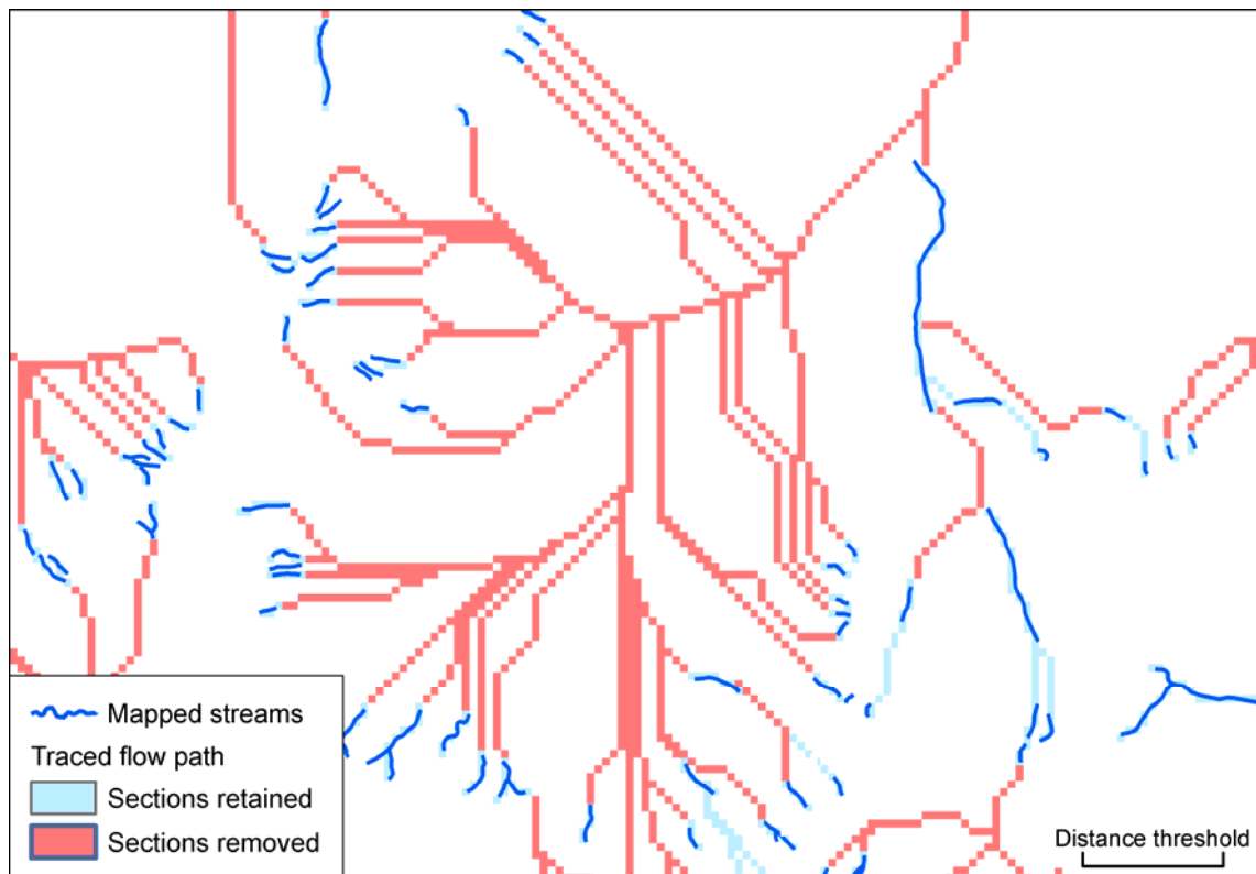
Figure 4.3 Delineating a stream network step 4: removing stream segments greater than a threshold flow path distance to a mapped streamline
