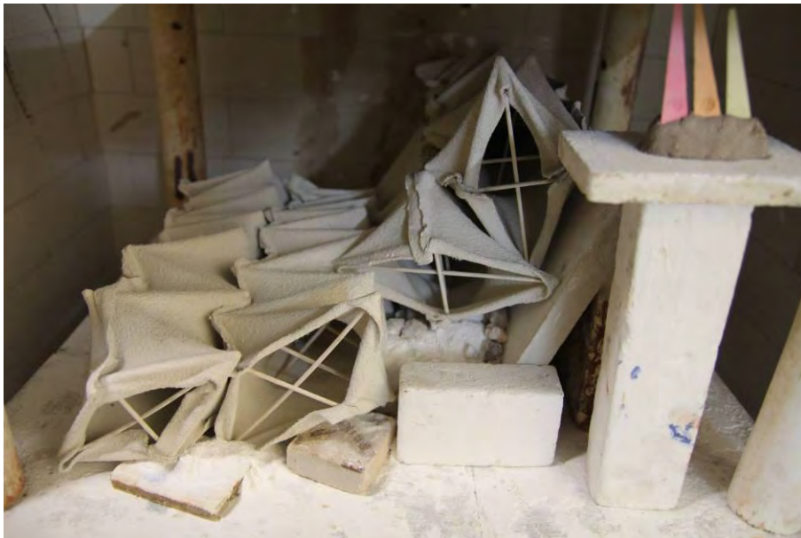
Fig. 113. Details of support method during firing type 2
