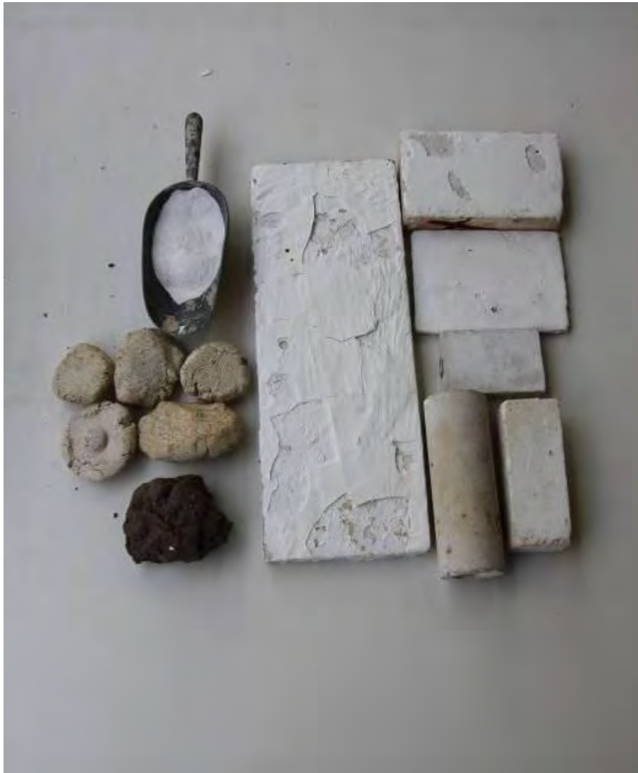
Fig. 111. Different support materials during firing
