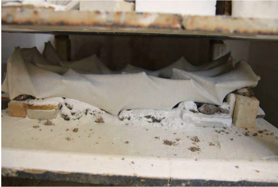
Fig. 112. Details of support method during firing type 1
