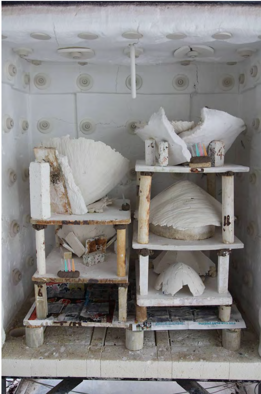
Fig. 110. Kiln packing type 3
