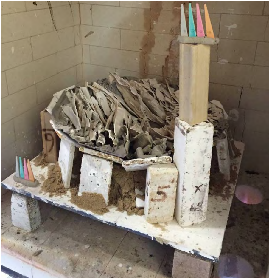
Fig. 109. Kiln packing type 2
