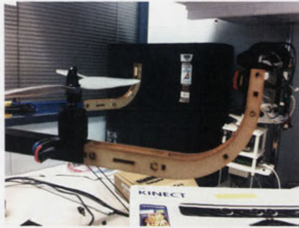
(b) Close-up view of safety support
