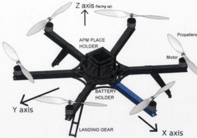
Figure 5.3: The hexacopter platform with its major components.
