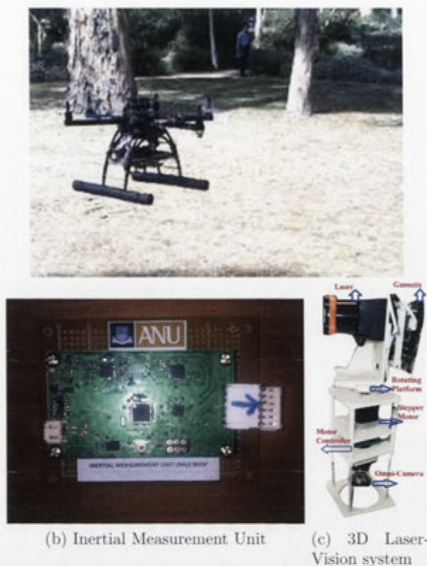
Figure 1.4: In-house developed hardware for SLAM applications. Please note that for the 3D Laser-Vision system, the interested readers are referred to our earlier work [57].
