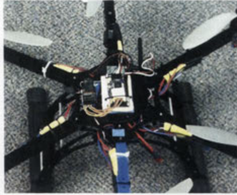
Figure 5.12: The autopilot was mounted onto the hexacopter platform and was placed on a the foam for vibration dampening.
