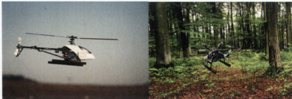
Figure 1.1: Aerial platforms (a helicopter and a hexacopter) developed in-house during this thesis, the helicopter is equipped with a PC104 and a Stereo Camera and an autopilot system. The hexacopter contains a Kinect and an in-house IMU as a payload with a dual-core Atom board.
