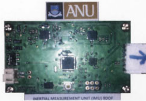
Figure 5.11: Inertial Measurement Unit developed for Visual-Inertial SLAM framework.
