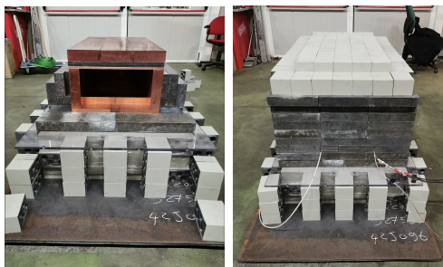
Figure 1. SABRE Hall B test setup with the external lead shield partially opened (left) and closed (right).
