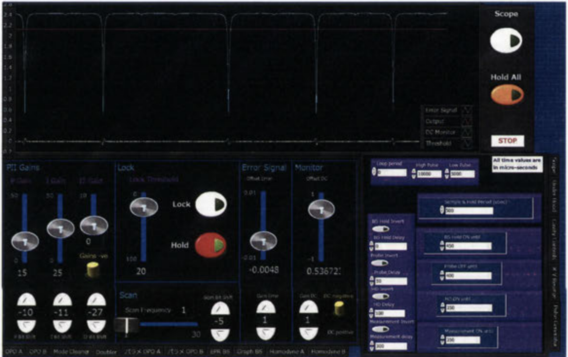
Figure 4.21: Front panel of Top_level.vi. All of the 10 phase locks as well as the TTL pulses are controlled here with an oscilloscope available for viewing the state of each phase lock.
