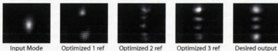
Figure 5.11: Progression of conversion from a TEM_{00} mode to a TEM_{30} mode. The CCD images after each reflection from the deformable mirror are shown. The final mode conversion resembles the desired output, but is not a perfect conversion. Source: [54].
