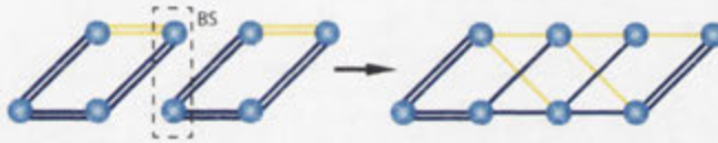
Figure 7.13: The dual-rail EPR-graph state G from sub-graphs. Upon interaction on a balanced beam-splitter (denoted by dashed box with BS label) the edge links in the sub-graphs are distributed to become weights of \pm\frac{1}{2} .
