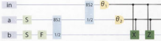
Figure 8.4: Teleportation-based computation through an EPR state with arbitrary homodyne measurements. All inputs are vacua. S : squeezing, F : Fourier, BS2 : beam-splitter with reflectivity \frac{1}{2} .
