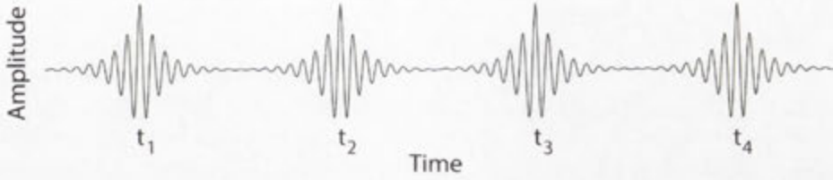
Figure 7.4: Pulsed light within continuous light. Pulses of light propagating within a continuous-wave beam.
