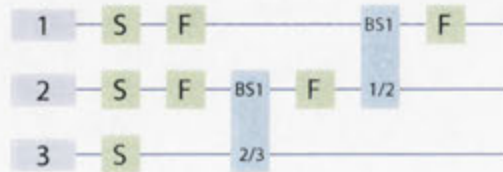
Figure 10.2: Generation of the 3-mode cluster state resource. Three squeezed modes are combined on two beam-splitters in order to generate a 3-mode linear cluster state. S : Squeezing operation, F : Fourier transform, BS1 : beam-splitter with reflectivity given by ratio indicated.
