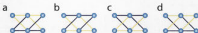
Figure 7.15: Polarity of edge weights as function of beam-splitter phase. There are four possible configurations of the polarities of the edge weights in graph G depending on which port of the beam-splitter sees the \pi phase shift.
