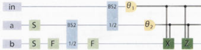
Figure 8.3: Teleportation-based computation through a cluster state with arbitrary homodyne measurements. All inputs are vacua. S : squeezing, F : Fourier, BS2 : beam-splitter with reflectivity \frac{1}{2} .
