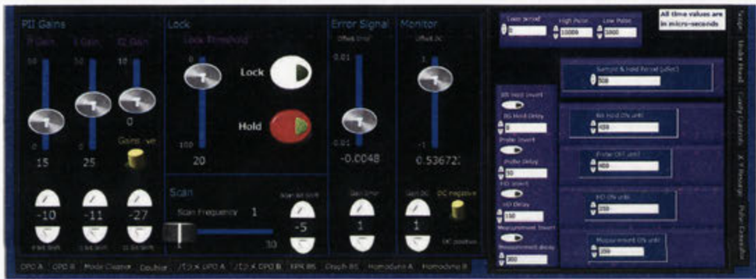
Figure 7.18: Portion of the control suite used to actively control ten optical systems.
