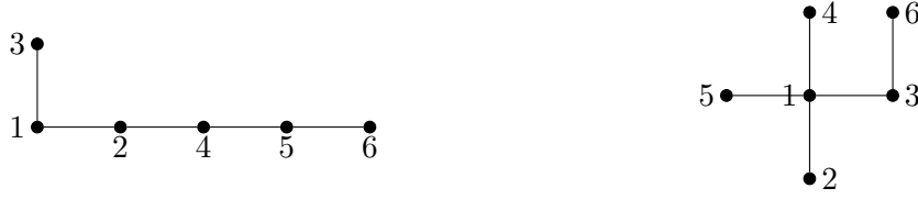
FIGURE 2.2: Two sampled graphs from the set of 1-connected graphs with |V| = 6 . Left: a 1-connected graph with low algebraic connectivity ( \lambda_2 = 0.081 ). Right: a 1-connected graph with high algebraic connectivity ( \lambda_2 = 0.485 ).
