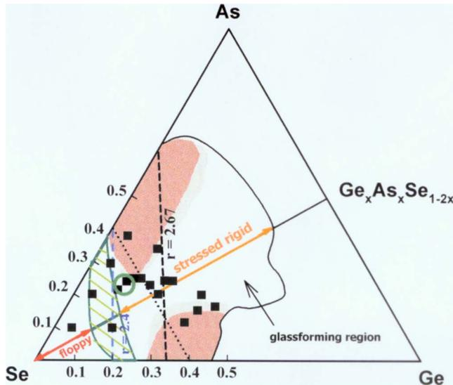
FIG. 1. (Color online) All our samples are marked in phase diagram of Ge–As–Se ternary glasses. The original phase diagram is provided by Professor Punit Boolchand. The intermediate phase is shown by the hashed region between the floppy and the stressed rigid phases. Nanophase-separated regions are shown by gray shading. Our best compositions with high nonlinearity and low optical loss are located at the green circle.
