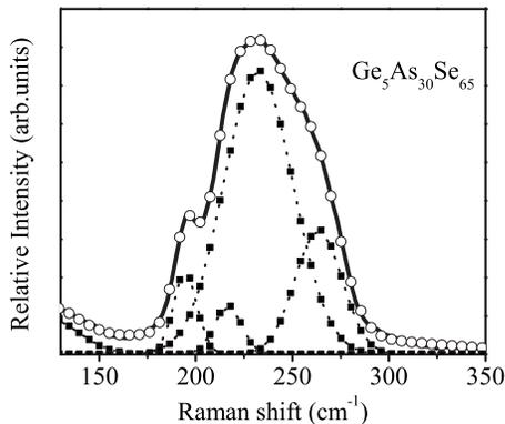
FIG. 3. The decomposed Raman spectrum for  $\text{Ge}_5\text{As}_{30}\text{Se}_{65}$  sample. The solid line is the experimental data, the open circles are the fitting spectrum, and the square-and-dotted lines are the decomposed Raman peaks.
