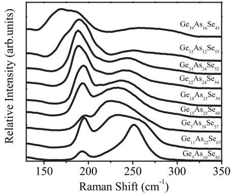
FIG. 2. Raman spectra of the typical glasses without the application of Bose–Einstein correction. The spectra are shifted along the  $y$ -axis in sequence from low to high MCN for clarification.
