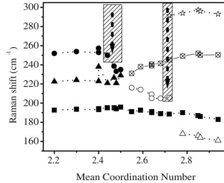
FIG. 4. Raman vibrational modes as a function of MCN. The different symbols represent different Raman vibrational modes that are described in the text. The shaded frames with the arrows indicate the regions of two transitionlike features.
