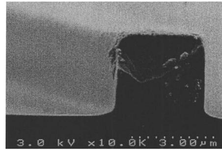
FIG. 4. Electron micrograph of 3  $\mu\text{m}$  wide waveguide etched in 20%  $\text{CHF}_3$  in oxygen mix at 10 mTorr, 20 W RIE power, and 200 W ICP power at 30 SCCM total gas flow.
