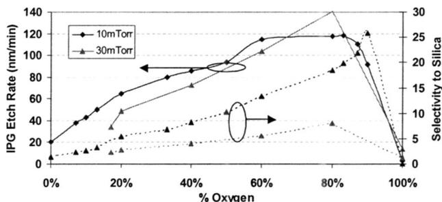
FIG. 3. Etch rate of IPG™ and selectivity to silicon dioxide in  $\text{CHF}_3/\text{O}_2$  gas mix.
