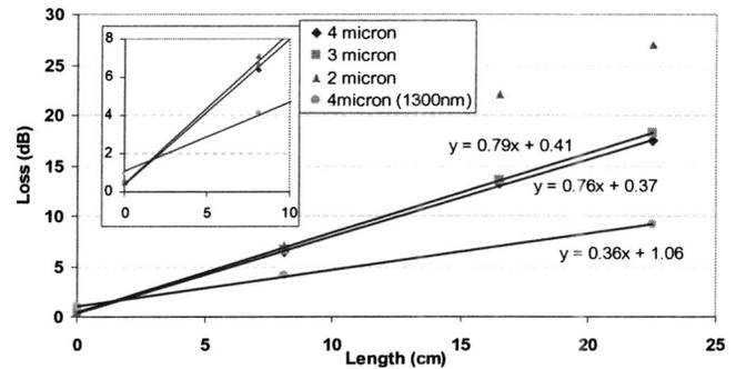
FIG. 6. Waveguide insertion loss data for nominal widths of 2–4  $\mu\text{m}$ . Lines are best linear fit to the raw data. The inset (b) is a magnified view of the 0–8 cm part of the graph showing loss variation as a function of the waveguide width.
