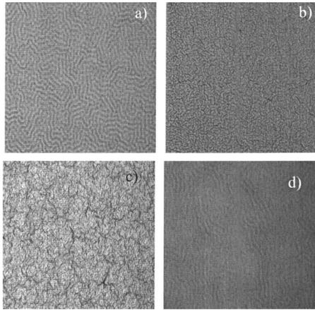
FIG. 1. Differential interference contrast optical microscope images of previously smooth aluminum films postbaking at 130 °C. Differing deposition conditions were used in (a)–(c). (d) shows the polysiloxane surface after the aluminum has been stripped revealing that the wrinkles have been permanently transferred to the polymer. Field of view is  $70 \times 70 \mu\text{m}^2$  in all images.
