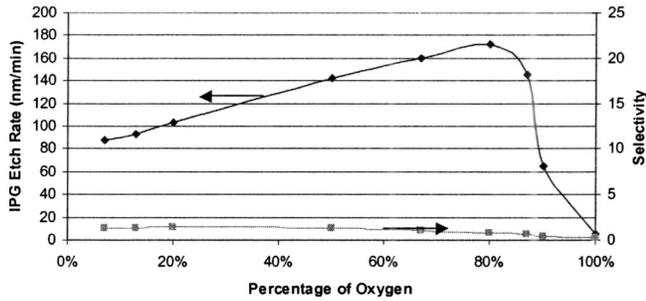
FIG. 2. Etch rate of IPG™ and selectivity against silicon dioxide in  $\text{CF}_4/\text{O}_2$  gas mixture.
