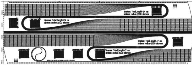
FIG. 5. Snake pattern layout schematic, inner bend radius was 2.5 mm, and outer radius was 3.2 mm.
