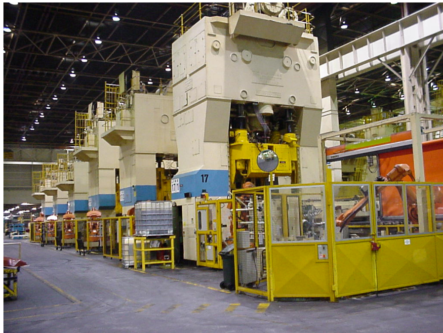
Figure 1: A line of heavy presses used in sheet metal forming.
