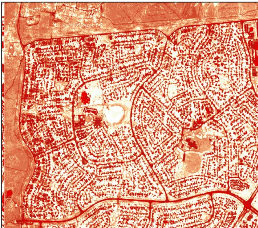
Figure 14: NVDI comparative distribution of built structures with 2002 above and 2006 below; red indicates the increase in reflective surfaces or built structures (SKM 2009).
