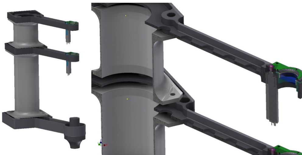
Figure 4. A close-up of the ADCs for one IFU. Each ADC consists of two rotating prism pairs with maximum clear aperture of 20mm.
