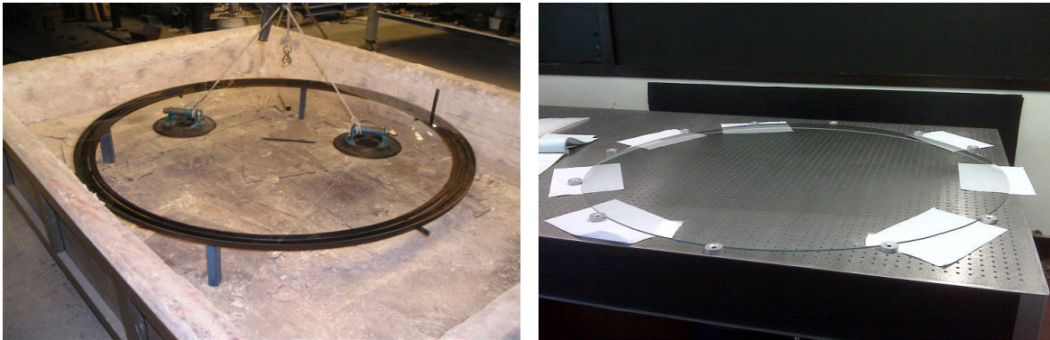
Figure 9: Prototype 1.3 m diameter Starphire GFP; (left) in furnace; (right) metrology test
