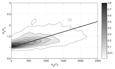
FIG. 6. Nondimensional decay as represented by (8) for all recorded altimeter measurements (212 cases). The solid line is for  $b_1 = 0.0014$ . The data consist of more than 23 000 individual data points. The data density is contoured with a max contour value of 1 and contours drawn at 0.01, 0.1, 0.2, 0.3, 0.4, 0.5, 0.6, 0.7, and 0.8.
