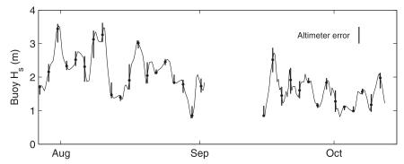
FIG. 4. The recorded buoy significant wave height (i.e.,  $H_s$ ) from location S1 of Young and Gorman (1995) at latitude 34°24′S. The vertical lines represent the span (from min to max) for a 30-h window across the data. Also shown is the typical altimeter measurement error (0.5 m).
