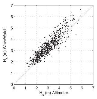
FIG. 3. Scatterplot comparing altimeter and WaveWatch-III estimates of the significant wave height (i.e.,  $H_s$ ). Comparisons are presented for each of 212 transects considered. The comparisons are presented at the "origin" point for each transect at approximately 40°S.
