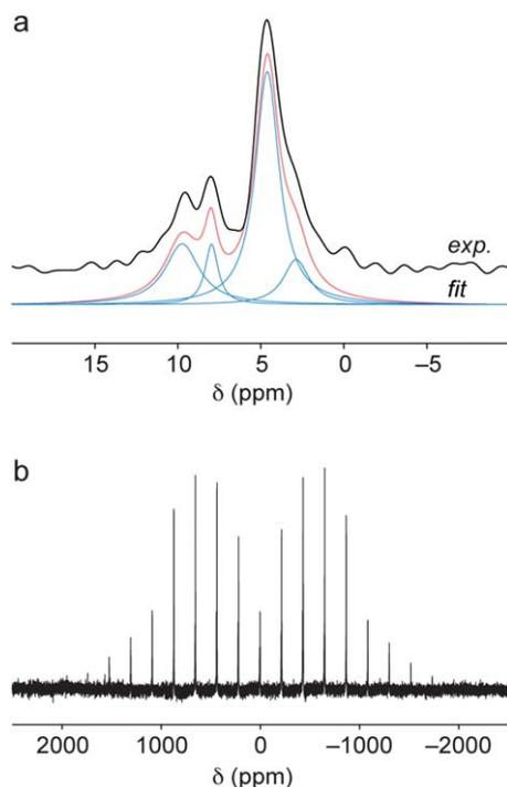
**Fig. 7** (a) Rotor-synchronised and (b) wide-spectral width  $^2\text{H}$  ( $14.1$  T) MAS NMR spectra of wads-D. A deconvolution of the experimental spectrum in (a) is shown below the MAS lineshape in red, with individual components shown in blue. Spectra are the result of coadding (a)  $4126$  and (b)  $12\,378$  transients separated by recycle intervals of  $5$  s. MAS rates were (a)  $12.5$  kHz and (b)  $20$  kHz.
