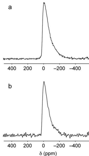
**Fig. 4**  $^{25}Mg$  (20.0 T) MAS NMR spectra of (a)  $^{25}Mg$ -enriched anhydrous wadsleyite and (b) wads-H. Spectra are the result of coadding (a) 109 552 and (b) 163 840 transients separated by a recycle interval of 0.5 s. For wads-H an initial DFS pulse was used to increase signal sensitivity. In both cases the MAS rate was 30 kHz.
