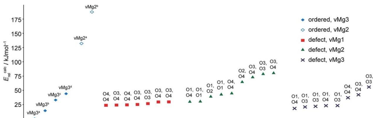
**Fig. 9** Calculated total energies for fully hydrated ordered model structures (represented by empty and filled blue diamonds) and structures containing a hydrated defect at an alternative cation site (represented by squares, triangles and crosses). For the defect model structures, the oxygen sites to which the hydrogen atoms are bonded within the alternative defect are indicated. Energies are shown relative to the lowest energy structure,  $\text{vMg3}^{\text{a}}$ .
