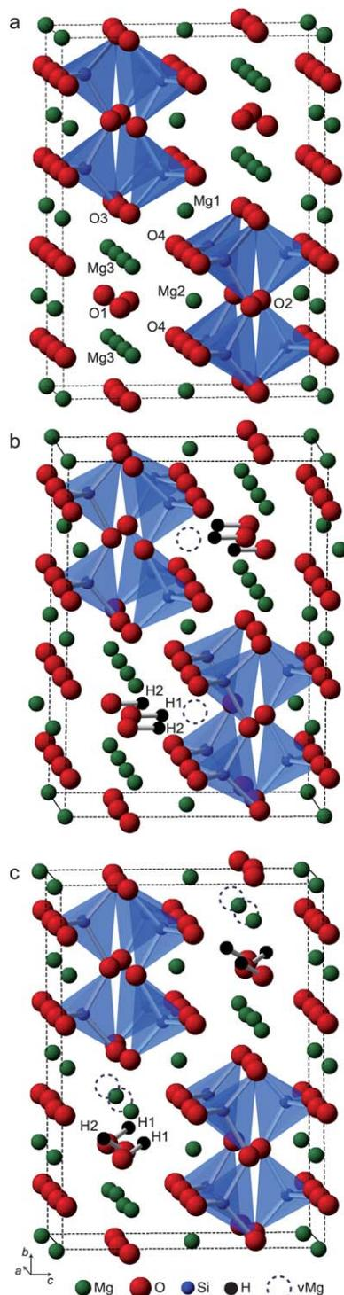
**Fig. 1** (a) Crystal structure of anhydrous wadsleyite with the four distinct O sites and three distinct Mg sites indicated. (b and c) Hypothetical ordered structures for fully hydrated hydrous wadsleyite obtained through full substitution of Mg2 and Mg3, respectively. Mg vacancies are indicated by dashed circles.
