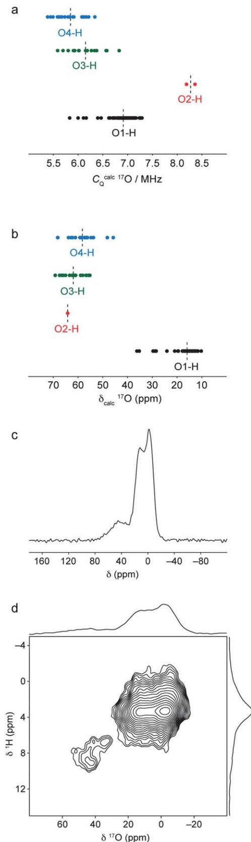
**Fig. 11** Calculated (a)  $^{17}\text{O}$  quadrupolar coupling constants and (b) chemical shifts for all O sites in the ordered and defect-containing model structures, grouped by local bonding environment. Average values for each group of parameters are indicated by dashed lines. (c)  $^1\text{H}$ - $^{17}\text{O}$  (20.0 T) CP MAS NMR
