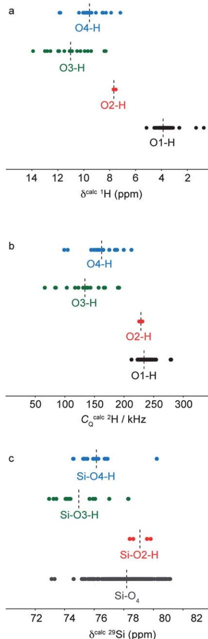
**Fig. 10** Calculated (a)  $^1\text{H}$  chemical shifts, (b)  $^2\text{H}$  quadrupolar coupling and (c)  $^{29}\text{Si}$  chemical shifts for all H and Si sites in the ordered and defect-containing model structures, grouped by local bonding environment. Average values for each group of parameters are indicated by dashed lines.
