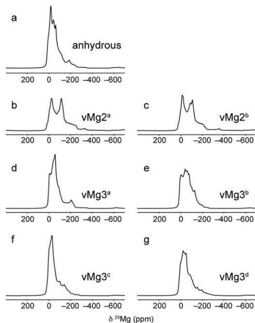
**Fig. 5** Simulated  $^{25}\text{Mg}$  (20.0 T) MAS NMR spectra for (a) anhydrous wadsleyite and (b–g) fully hydrated ordered model structures for hydrous wadsleyite based on calculated NMR parameters. In each case a Lorentzian line broadening factor of 400 Hz was applied prior to Fourier transformation of the simulated FID.
