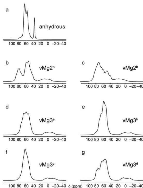
**Fig. 3** Simulated  $^{17}\text{O}$  (20.0 T) MAS NMR spectra for (a) anhydrous wadsleyite and (b–g) fully hydrated ordered model structures for hydrous wadsleyite based on calculated NMR parameters. Lorentzian line broadening factors of (a) 200 Hz and (b–g) 400 Hz were applied prior to Fourier transformation of the simulated FIDs.
