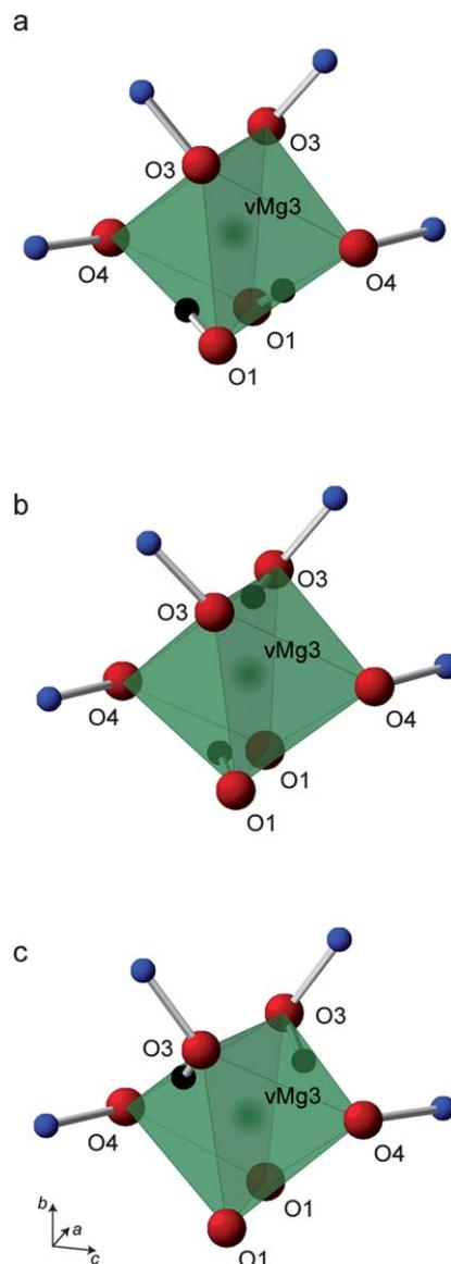
**Fig. 12** Expanded views of proposed models for hydrated defects surrounding the vacant Mg3 octahedron (shown in green) in the structure of hydrous wadsleyite. Vacancies are shown containing (a) two hydroxyl, (b) one hydroxyl and one silanol, and (c) two silanol protons. Oxygen, silicon and hydrogen atoms are represented by red, blue and black spheres, respectively. The nomenclature of the oxygen species is as given in the anhydrous crystal structure.<sup>10</sup>
