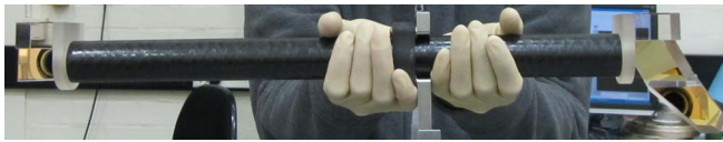
FIG. 1. Triple Mirror Assembly (TMA) designed by a consortium led by the Australian National University (ANU) and fabricated by the Commonwealth Scientific and Industrial Research Organisation (CSIRO). The mirrors TMA1 (left end of the tube) and TMA2, TMA3 (right end of the tube) are separated by 600 mm and aligned perpendicular to each other. The TMA is mounted by its bracket that is attached to the tube close to the center of mass.
