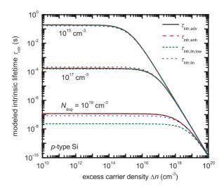
FIG. 9. (Color online) Intrinsic lifetime calculated with the parametrizations given in Eqs. (20)–(22) compared to the full parametrization of Eq. (18) for p-type Si.
