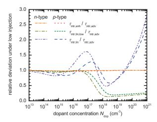
FIG. 10. (Color online) Relative deviation of the modeled intrinsic low-injection lifetime of Eqs. (20)–(22) with respect to the full parametrization of Eq. (18) for n-type and p-type Si.
