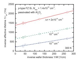
FIG. 2. (Color online) Plot of the inverse effective lifetime as a function of the inverse wafer thickness for Al<sub>2</sub>O<sub>3</sub>-passivated p-type FZ silicon samples with  $N_{\rm dop}=1.4\times10^{16}~\rm cm^{-3}$  and wafer thicknesses between 38 and 250  $\mu m$ . The data are shown exemplarily for three different excess carrier densities  $\Delta n$ .
