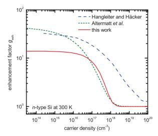
FIG. 8. (Color online) Enhancement factor  $g_{\text{eeh}}$  for lowly injected n-type silicon. The experimentally quantified  $g_{\text{eeh}}$  of Altermatt et al., Eq. (4), and this work, Eq. (19), are compared to the theoretically determined  $g_{\text{eeh}}$  of Hangleiter and Häcker (Ref. 12).
