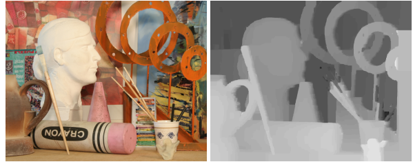
Figure 3. The drifting of the depth boundaries fattens and shrinks areas of homogeneous depth. The right image is a depth map produced by \alpha -expansion. The brush next to the jar becomes thicker, whereas the sticks in the cup partly disappear. Blurry boundaries are quite common.
