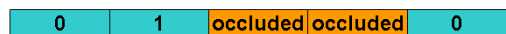
Figure 4. Five horizontally continuous pixels on the right image are labeled as above. The disparity range in the problem is between 0 and 1. Whereas two pixels are labeled as occluded, only the left one can be occluded.
