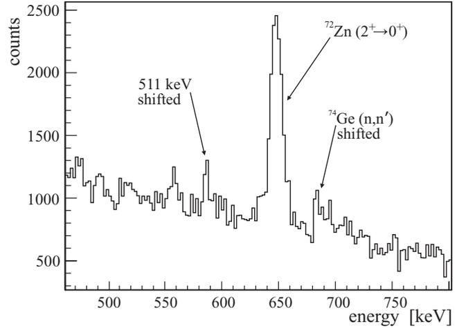
FIG. 3. Doppler-corrected random-subtracted  $\gamma$ -ray spectrum near the  $^{72}\text{Zn}$  ( $2^+ \rightarrow 0^+$ ) line. This spectrum represents all of the data for the pair of clover crystals at  $148^\circ$  with respect to the beam axis in Run IV.
