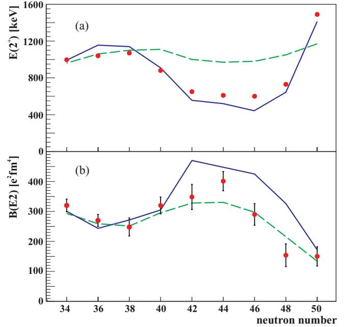
FIG. 7. (Color online) Energies of the  $2^+$  states (a) and transition probabilities  $B(E2; 2^+ \rightarrow 0^+)$  (b) of the Zn isotopes. Filled circles: experimental values, dashed lines: JUN45 interaction [8], solid lines: LNPS interaction [9]. Effective charges of ( $e_p = 1.5$ ;  $e_n = 1.1$ ) and ( $e_p = 1.5$ ;  $e_n = 0.5$ ) were used, respectively, for the calculation in the JUN45 and LNPS interactions.
