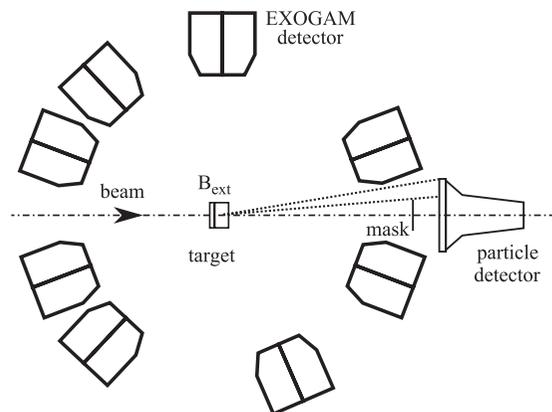
FIG. 1. Experimental setup, from above. The beam traverses the target and is detected in the forward direction. The target is polarized by an external magnetic field  $B_{\text{ext}}$  directed perpendicular to the page. The de-excitation  $\gamma$  rays are detected by eight EXOGAM detectors.
