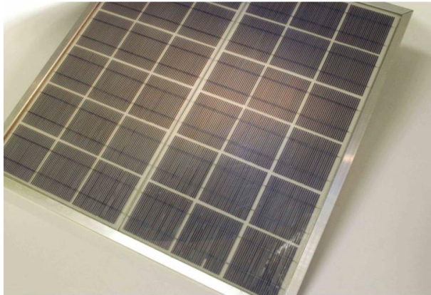
Figure 12. A Sliver module constructed from Raft sub-modules.
