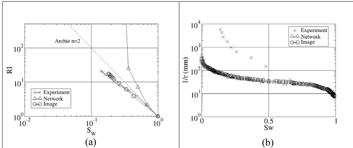
**Fig-7:** Comparison of (a) resistivity index and (b) capillary entry radius for the Middle Eastern carbonate reservoir sample.
