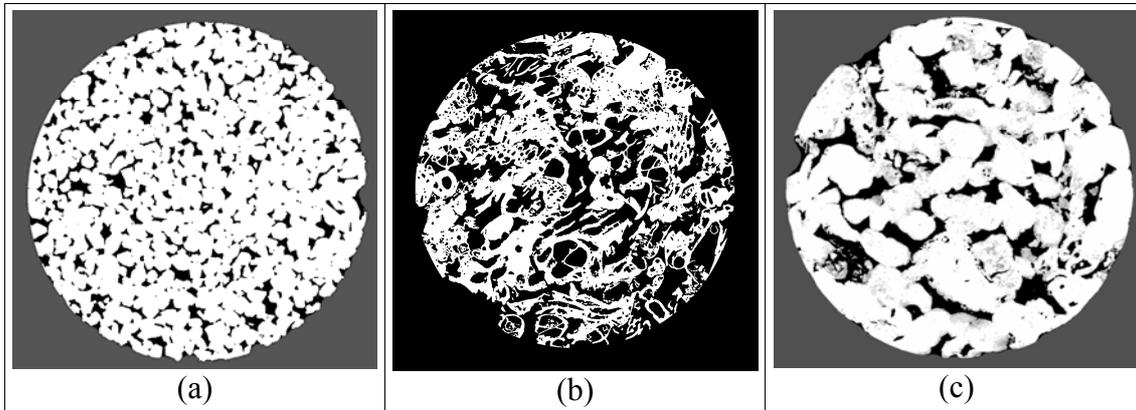
**Fig-1:** Micro-CT images of (a) Fontainebleau (b) Mt. Gambier and (c) Middle Eastern Carbonate.
