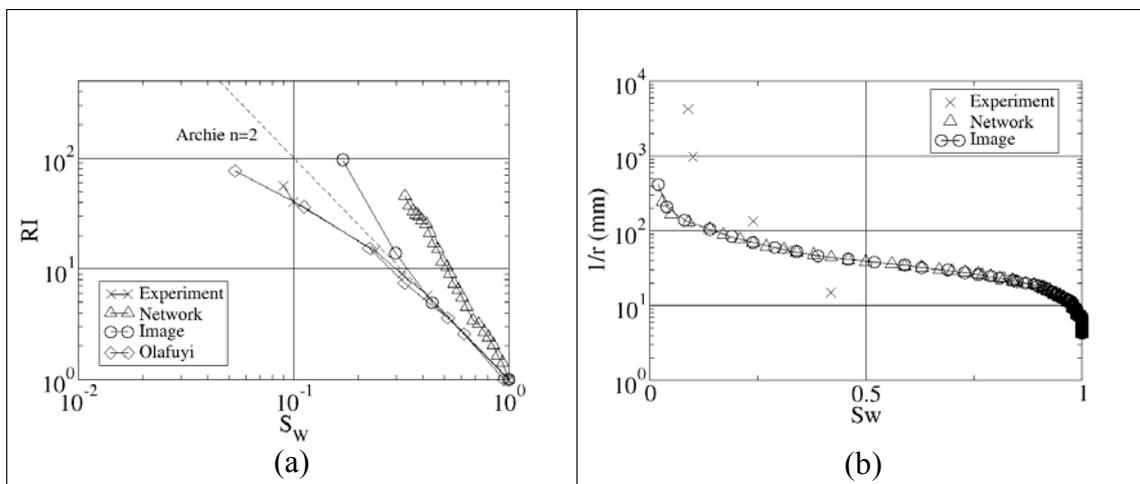
**Fig-6:** Comparison of (a) resistivity index and (b) capillary entry radius for the Mt. Gambier sample.
