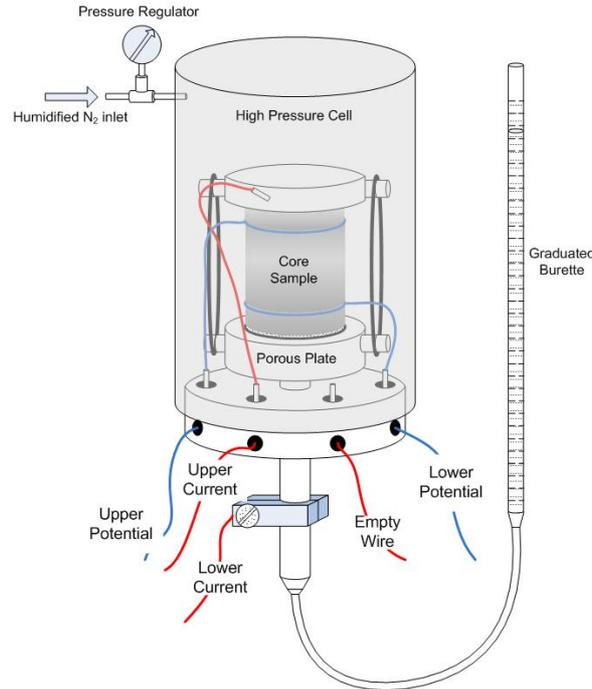
**Fig-2:** The porous plate technique for resistivity index and capillary pressure measurement.
