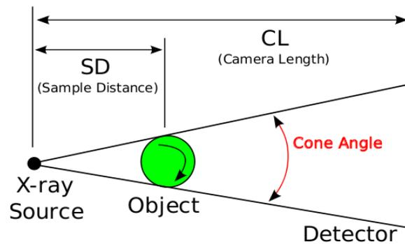
**Fig-3** Experimental X-ray CT apparatus.
