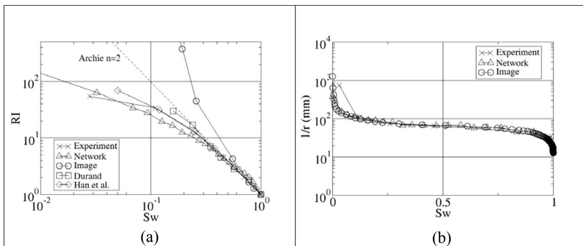
Fig-5: Comparison of (a) resistivity index and (b) capillary entry radius for the Fontainebleau sample.
