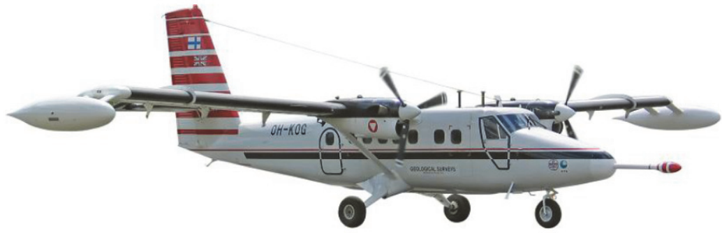
Figure 1.4 The GTK-AEM-05 frequency-domain AEM system which has pods mounted on the wing tips that house the transmitter and receiver coils.
