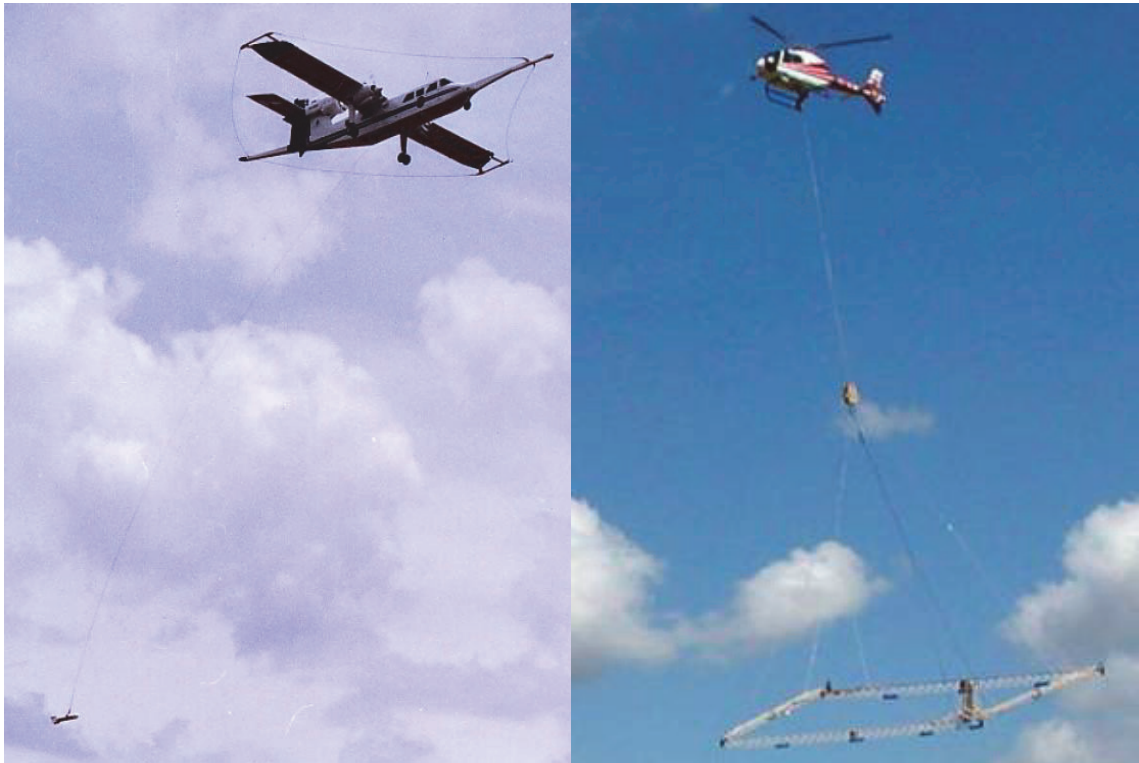
Figure 1.7 Examples of time-domain AEM systems. The left hand panel shows an early TEMPEST system aircraft carrying a wire transmitter loop (slung between the wingtips, tail and nose), and towing the receiver bird (bottom left of photograph). The right hand panel shows the SKYTEM system in which a frame, that carries both the transmitter loop and receiver coils, is towed below a helicopter.
