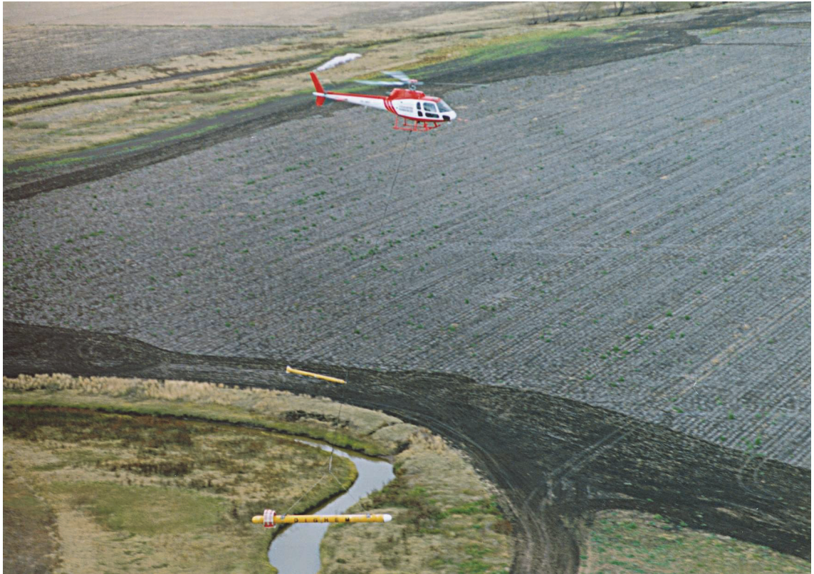
Figure 1.3 Photograph of the DIGHEM frequency-domain AEM system that shows a magnetometer bird (top) and electromagnetic bird (bottom) that is towed approximately 30 m below the helicopter.
