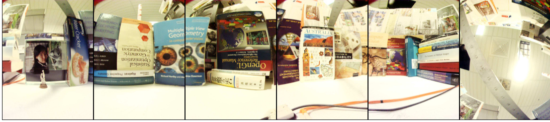
Figure 8.13: Experiment setup with a Ladybug™2 camera and books surrounding the camera. The Ladybug™2 camera is placed on a piece of A2-size paper on which the trajectory of 108 positions of cameras is printed.
