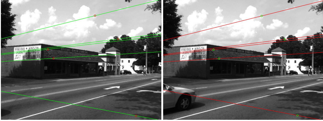
Figure 7.11: Five points selected from the left-backward camera in two views, frame 120 and frame 125. Epipolar lines corresponding the five points are plotted. An essential matrix is estimated from the selected five points. The five points from the first view is indicated as red circles and the five epipolar lines corresponding to the five points are shown as red lines in the second image. In the same way, green circles for 5 points in the second view and green lines for the corresponding epipolar liners.
