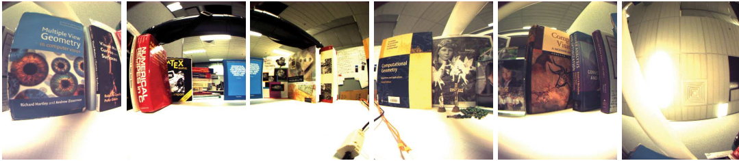
Figure 10.10: Six images captured at each camera of LadyBug. Five cameras (camera id 0 to 4) are placed to look horizontally view, and the last one (camera id 5) is located for a top view (From left to right order). There are only small overlapped fields of view across cameras.
