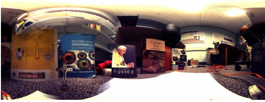
Figure 9.3: A panoramic image is obtained by stitching together all six images from the Ladybug TM 2 camera. This image is created by LadybugPro, the software provided by Point Grey Research Inc.
