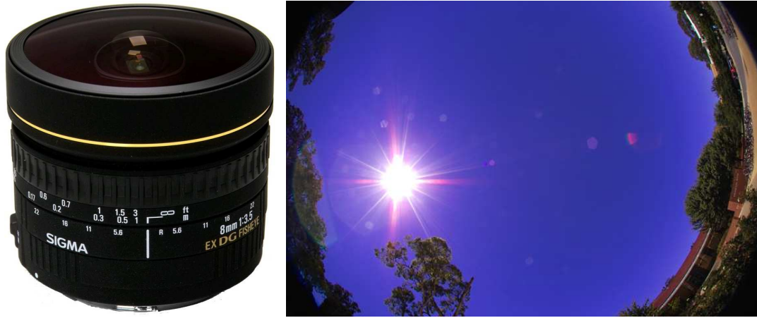
Figure 4.6: Dioptric imaging system. Sigma 8 – mm fisheye lens for a DSLR camera and the photograph taken by a Sigma SD9 camera with the fisheye lens. Dioptric camera systems have a lens with a wide field of view to obtain a large field of view. The lens is a concave lens so as to capture a large number of incoming light rays. (Photograph by Jae-Hak Kim)
