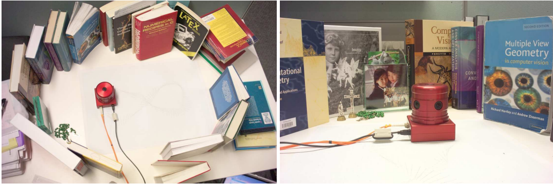
Figure 10.9: Experiment setup. A LadyBug camera is placed on a piece of paper which has 1mm grids and it is surrounded by books. A trajectory of cameras is marked on the paper. Total 108 positions of ground truth are measured from the marked positions.
