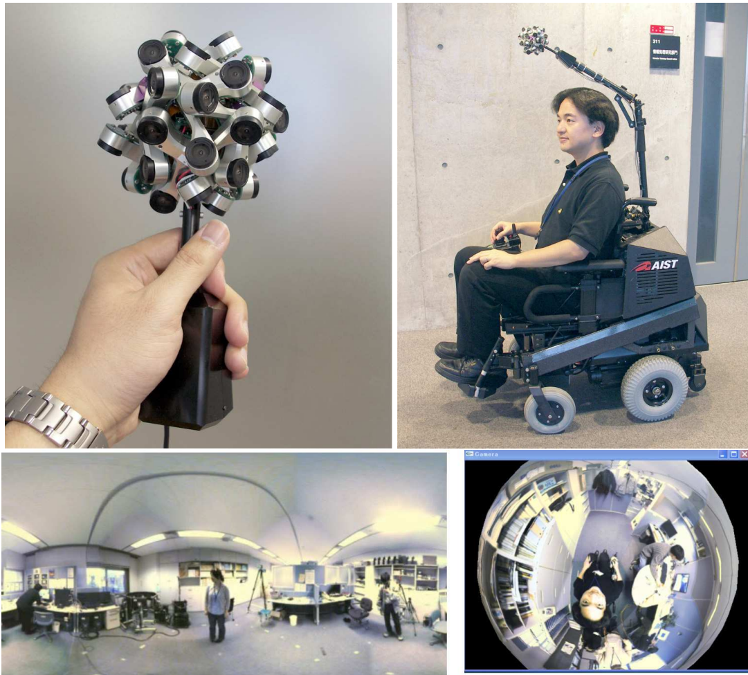
Figure 4.7: Camera cluster. The Stereo Omnidirectional System (SOS) by Japan's National Institute of Advanced Industrial Science and Technology and developed in collaboration with the National Rehabilitation Center for Persons with Disabilities. It provides not only omnidirectional images but also depth from stereo for people using wheelchairs. (Copyright ©National Institute of Advanced Industrial Science and Technology (AIST), Japan. All rights reserved. Reprinted with permission from AIST).
