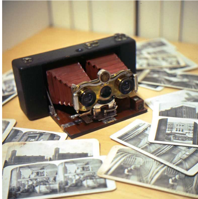
Figure 3.1: Stereo camera and photographs taken by the stereo camera: Kodak Brownie Hawkeye Stereo Model 4, manufactured between 1907 and 1911. (Courtesy of Timothy Crabtree from www.deviantart.com , All copyrights reserved ©2008. Reprinted with permission.)
