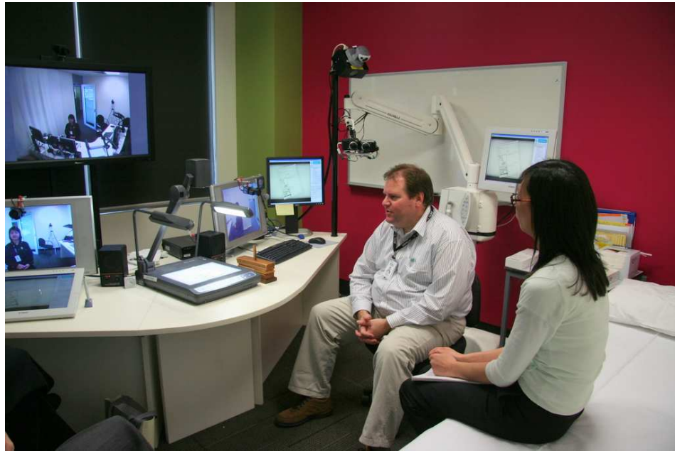
Figure 9.4: Patient's room showing the correspondence of the two close-up displays and the room overview display from the surgeon's room.
