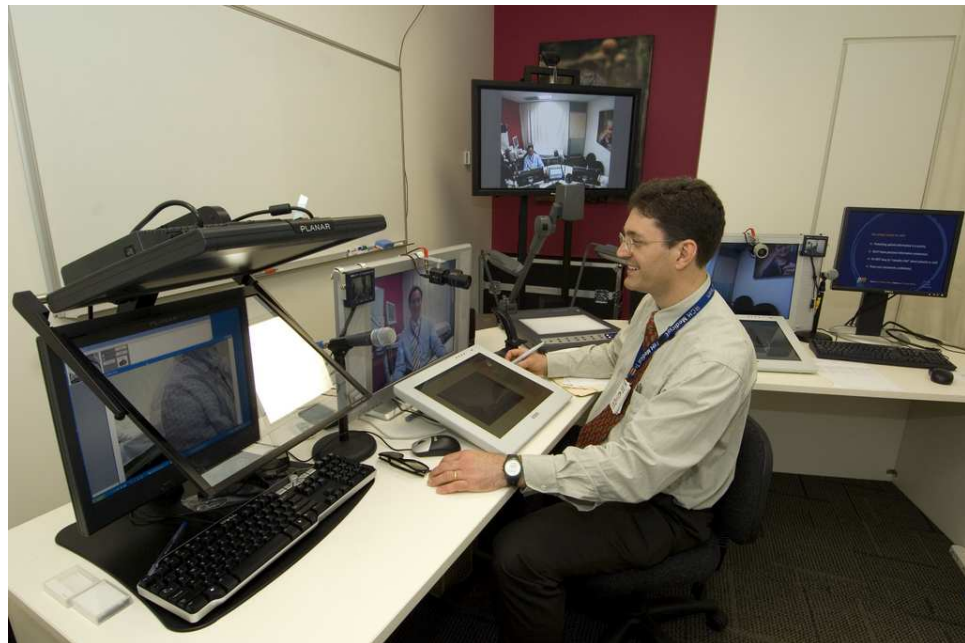
Figure 9.4: Surgeon's room. From left to right: 3D display, examination close-up subsystem, document scanner (below) and patient's room overview (above), consultation close-up subsystem and hospital computer monitor (Photo courtesy Royal Children's Hospital)
