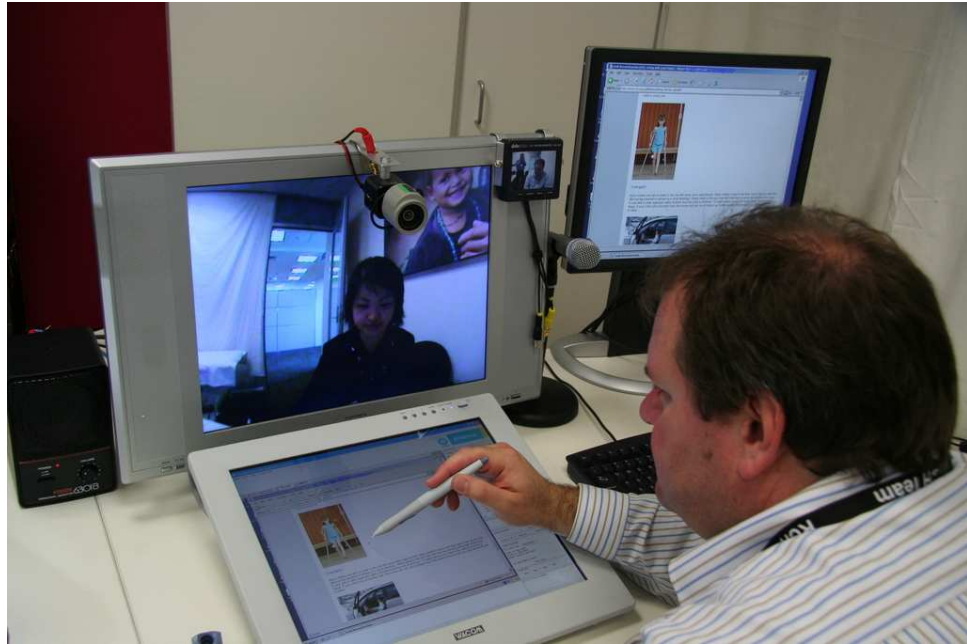
Figure 9.2: Close-up video/audio subsystem with tablet and pen display
