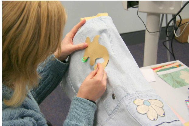
Figure 7.6: Placing a fabric patch on the dress. In workspace guidance mode the green laser cursor (below her left thumb) shows the required position of the patch directly in the workspace
