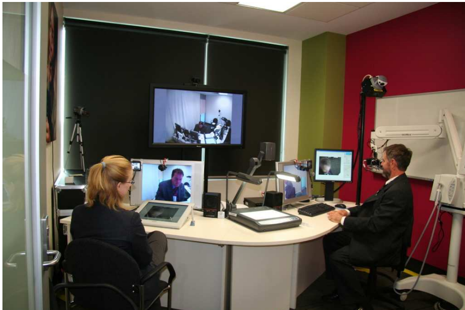
Figure 9.3: Patient's room. The pole camera is above the person sitting on the right, the arm-mounted cameras are by his head, the hand-held camera is on a flexible cable behind him and the examination close-up camera is in front of him. The document scanner is on the desk.
