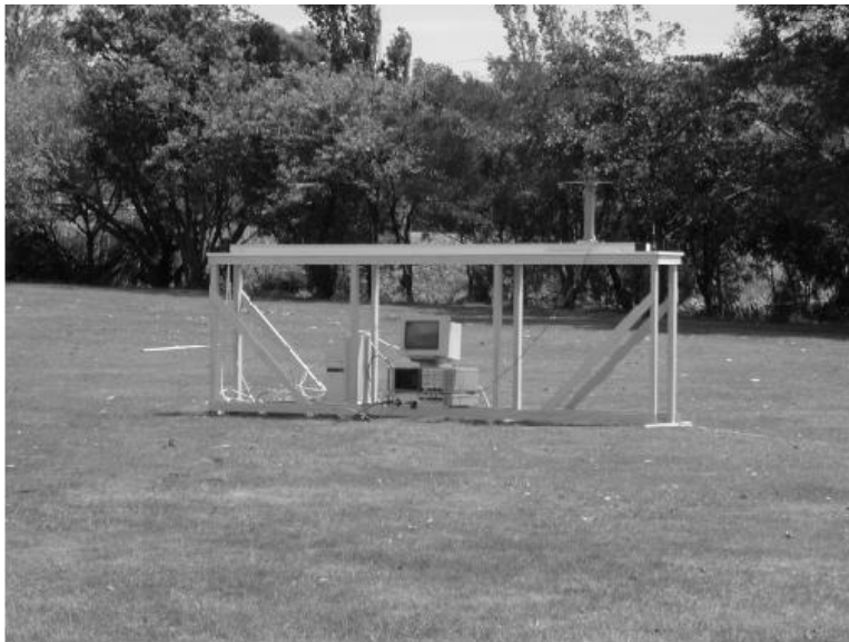
Figure 4.9: The synthetic receiving array outdoors. The monopole is in the centre of a circular ground plane. The network analyser and servo control apparatus are located under the table.
