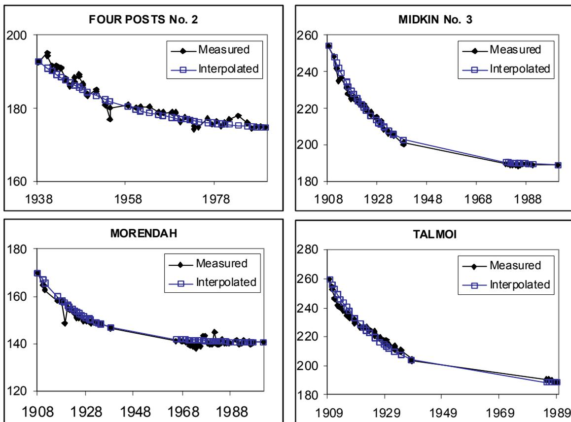
**Figure 2 Measured and interpolated water levels for some bores with long datasets. Interpolated values use equation (1) with  $\alpha=0.00014$  and are based only on the first and last measurements of each bore.**
