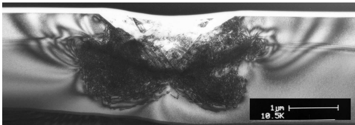
Figure 4.12: Bright-field TEM images of indent in 100 nm layer of \text{SiO}_2 containing Si-nc with maximum load of 100 mN. The oxide layer remains intact.
