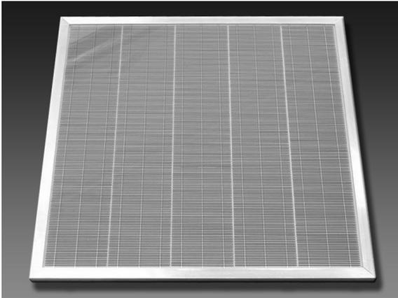
**Figure 5:** 1000cm<sup>2</sup> Sliver® module. The cells are spaced at double their width and the module has a rear Lambertian reflector.
