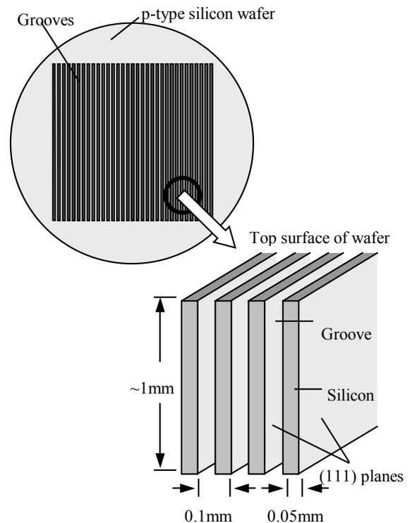
**Figure 1:** Sliver® wafer. Long thin silicon slices are supported by the wafer frame.
