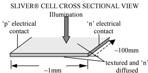
**Figure 2:** Schematic of the Sliver® cell design.
