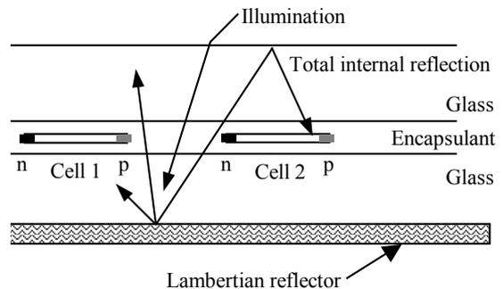
**Figure 3:** Lambertian reflector module design. The small width and bifacial nature of the Sliver® cell enables the cells to be spaced out (in this case double cell width, halving silicon use).
