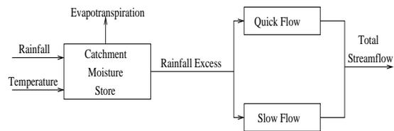
**Figure 1:** Basic structure of the IHACRES model
