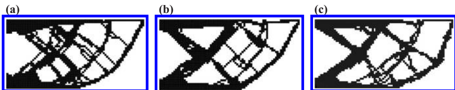
Figure 13. Optimal topologies of structure with isotropic material but different growth speeds ( g_2 = 1.25g_1 ) and initial designs ( \rho^{(1)} )
