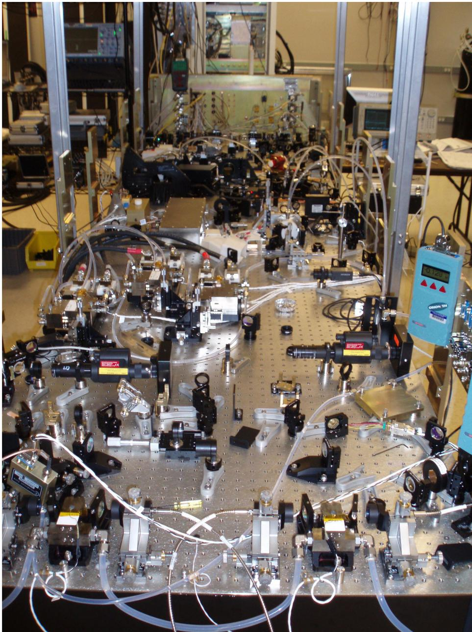
Figure 7: Gemini South laser bench with 1319 nm oscillator in foreground
