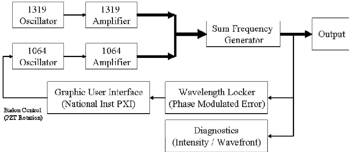
Figure 1: GLS block diagram
