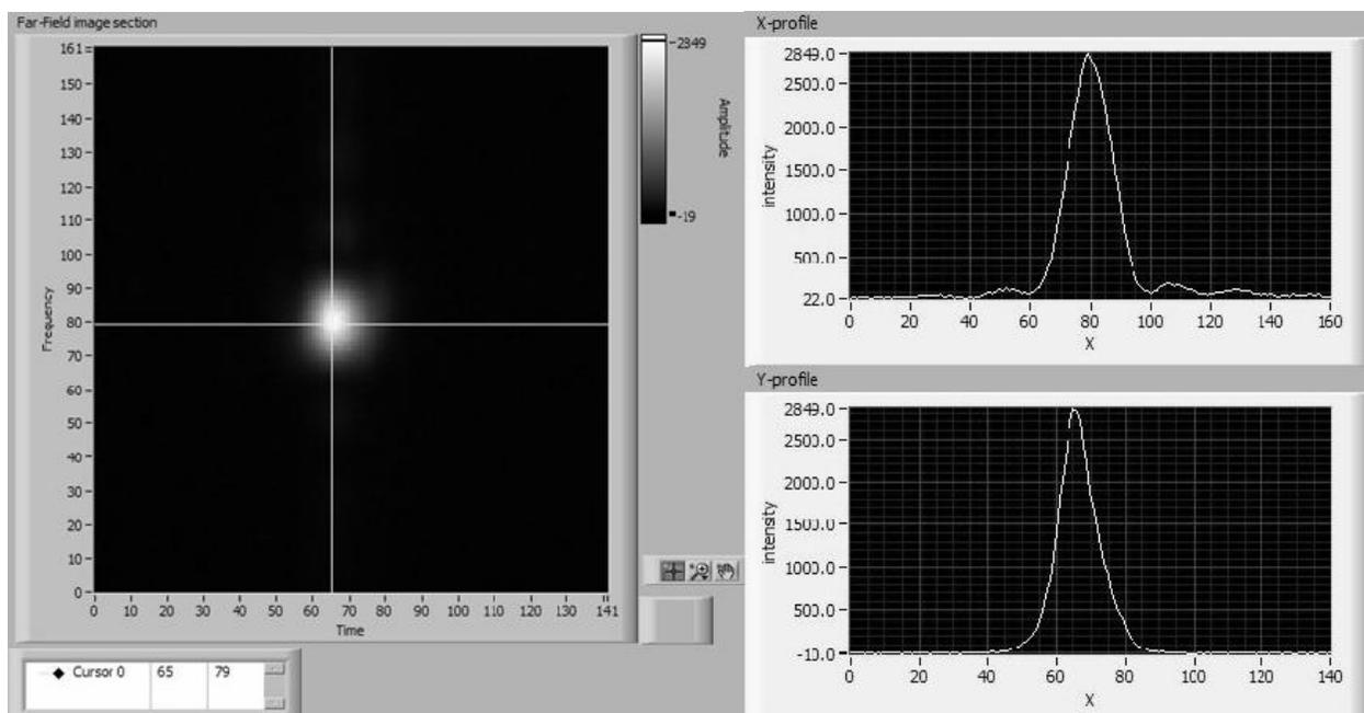
Figure 4: Far field profile, 76 W at 1319 nm
