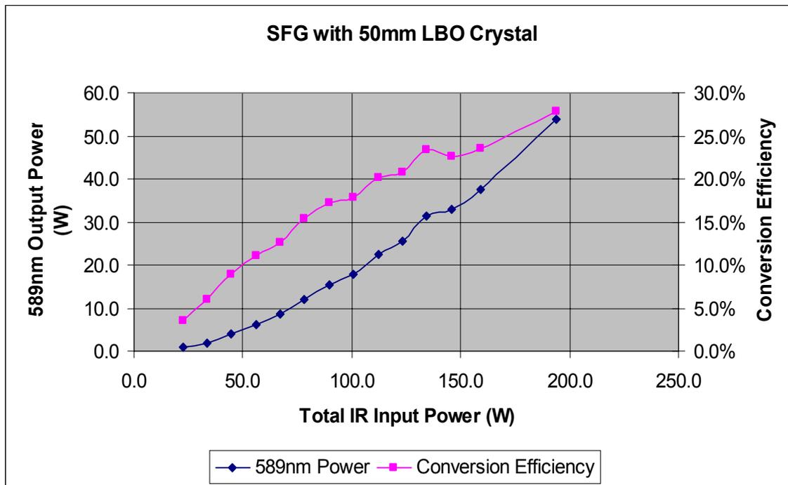
Figure 5: 589 nm power and conversion efficiency vs. IR input
