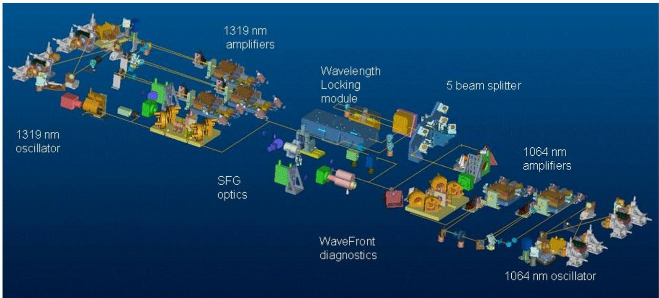
Figure 3: Gemini South laser system optical layout
