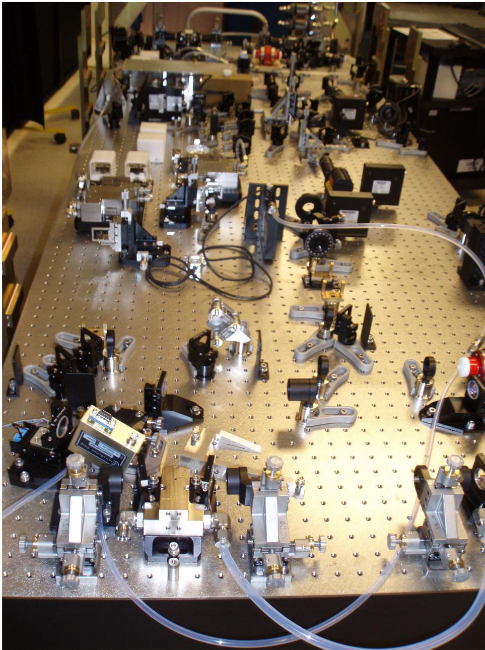
Figure 9: Keck I laser bench with 1319 nm oscillator in foreground
