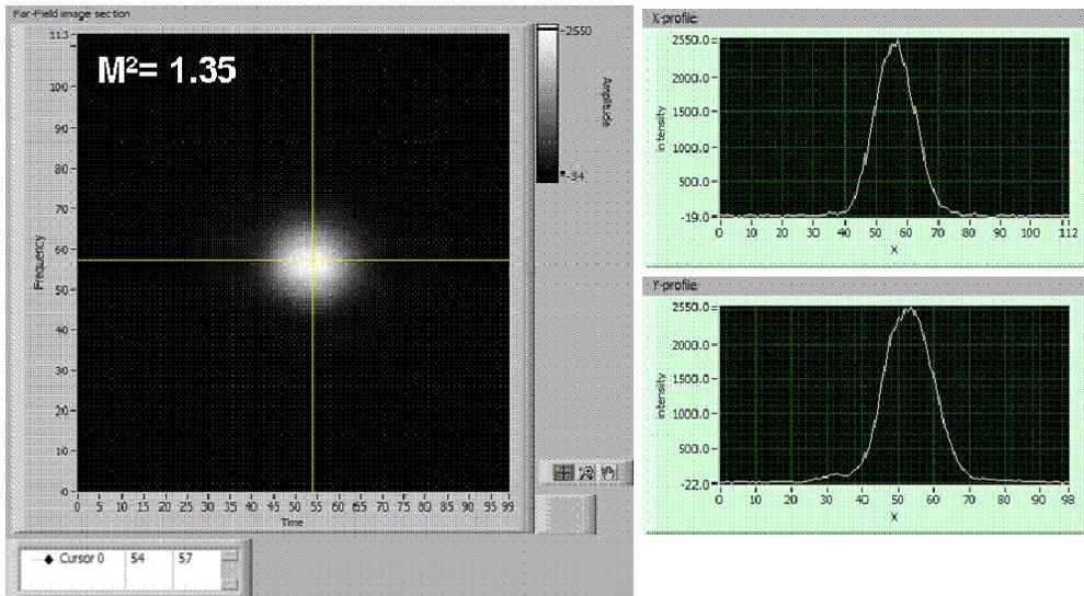
Figure 6: Far Field Beam quality data for the Keck I GLS
