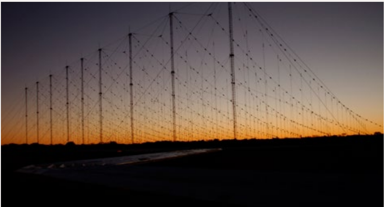
A Jindalee Operational Radar Network (JORN) transmitter site at sunset, Harts Range, Alice Springs. JORN is an over-the-horizon radar network that can monitor air and sea movements across 37,000 km 2 . Photo courtesy Department of Defence.
