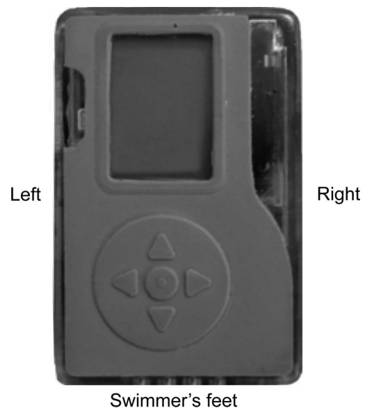
Figure 1. Inertial sensor package (MiniTraqua™) used to quantify kick count and kick rate. The image is presented to scale and is orientated as it appeared on the thigh and shank during testing.
